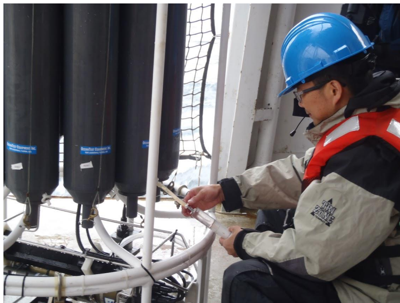
Figure 8. Water sampling for methane measurements using the CTD-rosette.
