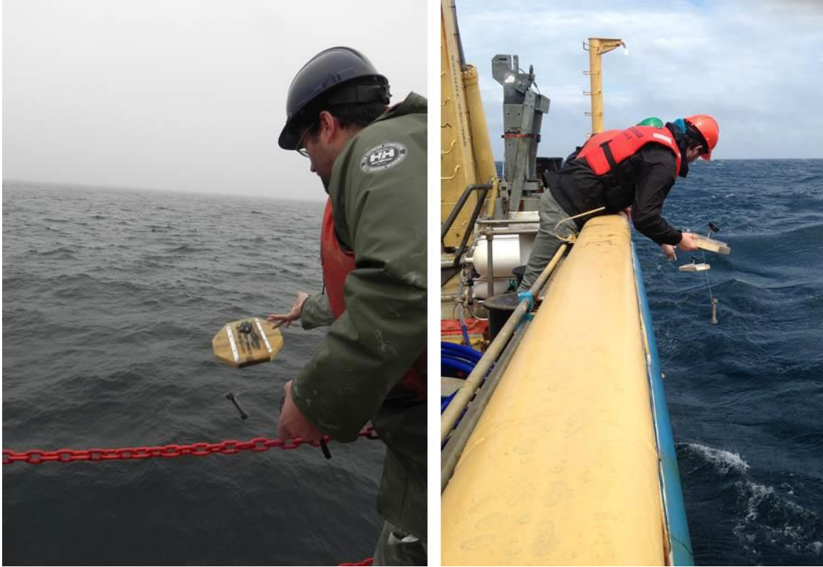
Figure 7. GPS(Spot)-emitting drifters deployment.
