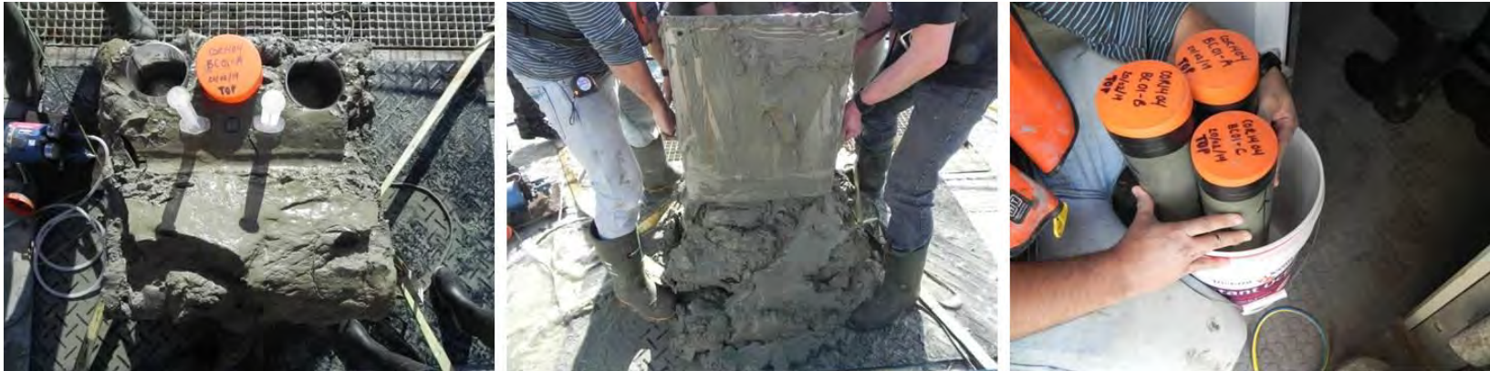
Figure 105. COR1404_001BC pictures. From right to left: sample from top, side and the push cores.
