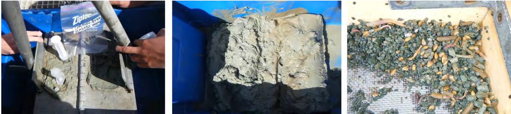
Figure 85. COR1404_BV44 pictures. From right to left: sample from top, opened, and sieved for benthic organisms.
