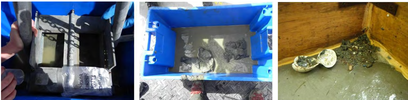
Figure 54. COR1404_BV13 pictures. From right to left: sample from top, opened, and sieved for benthic organisms.
