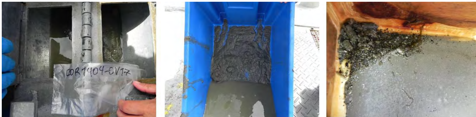
Figure 58. COR1404_BV17 pictures. From right to left: sample from top, opened, and sieved for benthic organisms.
