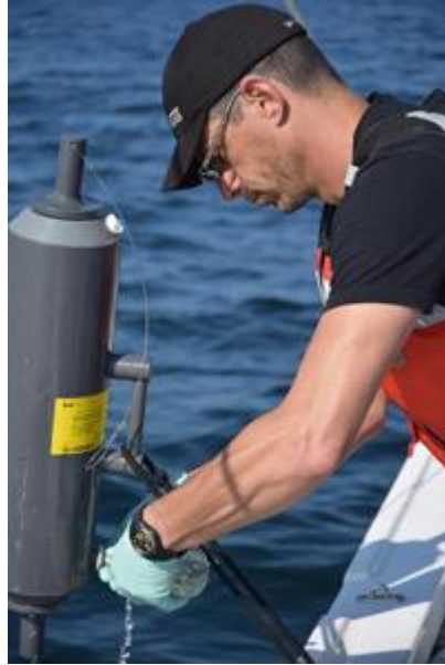
Water sample taken to measure the concentration of dissolved oxygen
