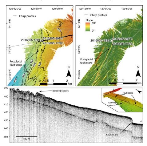
Figure 35.4. Fault scarps recognized in 2015 and further investigated in this cruise.
