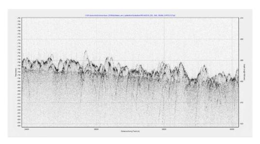
Figure 38.7 ub-bottom profile at point in site ROV 4 (black dot in Figure 38.6) showing potential unconformity between highly rugose surface features and harder reflector below.
