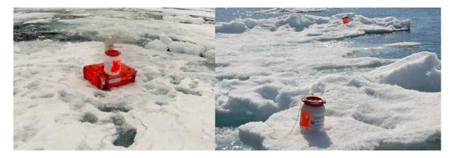
Figure 4.2. Deployment of the Aquadopp on an ice floe, within the MIZ (left panel), and the wave buoys alone (right panel).
