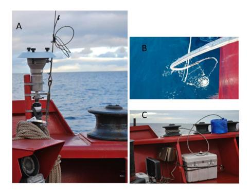
Figure 28.5. A) Air Sampler on the bow of the *Amundsen* collecting Arctic air in 48 hour intervals. **B-C)** Submersible pump collecting surface water at the bow into containers on the deck.
