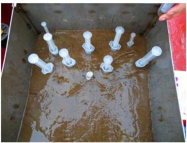
Figure 32.1. Box core deployment and sediment cores sampling.
