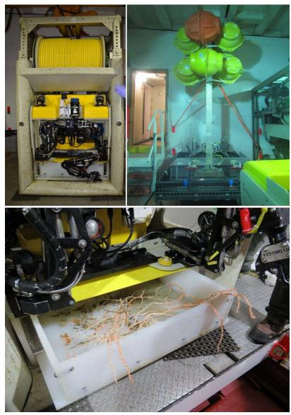
Figure 38.2 A) Super Mohawk (SuMo) ROV, B) elevator, and C) sampling skid with Keratoisis sp. samples.
