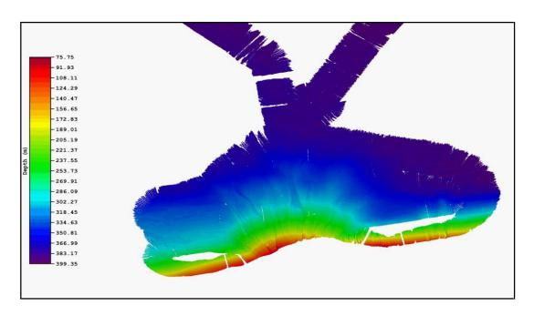
Figure 33.11. Bathymetric coverage of Ballast Fan showing many channels occupied by cyclic steps.
