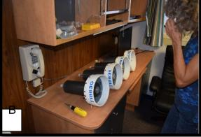
Figure 9.8 Sediment trap timers All timers were set simultaneously and turned on at the exact same time at 0:00 Hr on 4-October-2016.
