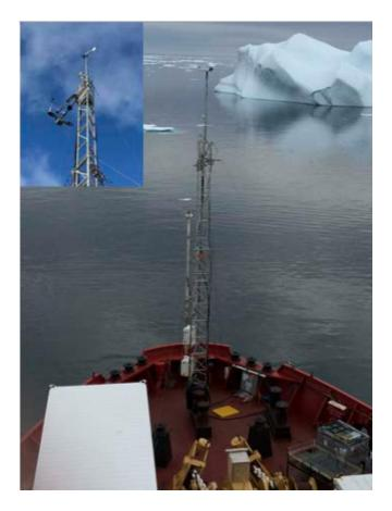
Figure 2.2. Meteorological tower located on the foredeck of the Amundsen with EC flux system (inset).
