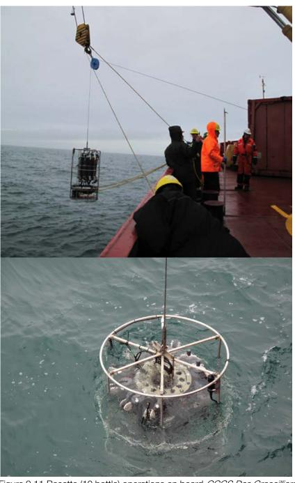
Figure 9.11 Rosette (10 bottle) operations on board CCGS Des Groseilliers
