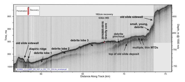
Figure 35.3. Debrite deposits (gravity mass wasting debris) situated within a large, older slide complex and partially covered with post-glacial stratified sediments.
