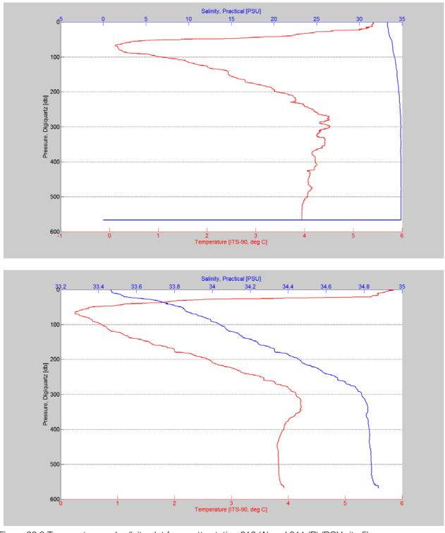
Figure 38.9 Temperature and salinity plot for rosette station 010 (A) and 011 (B) (ROV site 5)
