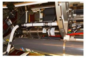
Figure 10.23. UVP mounted on the bottom of the SBE32 caroussel on the Amundsen
