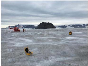
Figure 3.9. Making ground-penetrating radar measurements of ice thickness on Mittie Glacier, Manson Icefield, August 16, 2016 (N76° 53.732', W78° 58.774'). Ice thickness at this location was ~220 m. Photo courtesy of Luke Copland.
