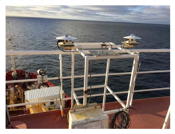
Figure 2.1. The radiation sensors and digital camera ocated above the wheelhouse of the Amundsen. Shown are the pyrgeometer (left), pyranometer (right) and PAR sensor (centre). The automated digital camera is mounted on the rail below and to the left of the prygeometer.
