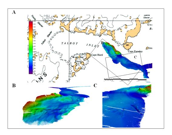
Figure 33.9. A) Bathymetric coverage inside Trinity Fjord; B) Horizontal 3D image of the glacial lineation on the seabed; C) Iceberg scours.
