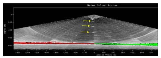
Figure 33.33. Caris Water column display used to assess the position and depth of BR-1-16 mooring. Yellow arrows show the buoys in the water column.
