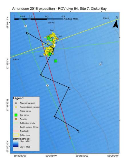
Figure 38.22 Map of site 7 (Disko Fan, Dive 54) showing planned and accomplished ROV transect during the 2016 CCGS Amundsen expedition. A and B indicate subbottom profile positions shown in figure 21
