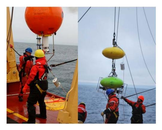
Figure 28.1. SPMD cage installed on the mooring line on BREA mooring BR-3 (left) and BR-K (right).
