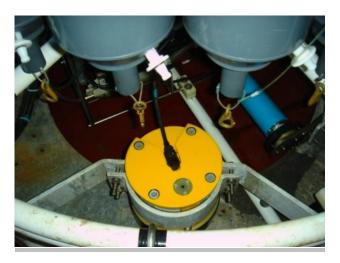
Figure 10.20. RDI LADCP mounted on the bottom of the SBE32 caroussel on the Amundsen.
