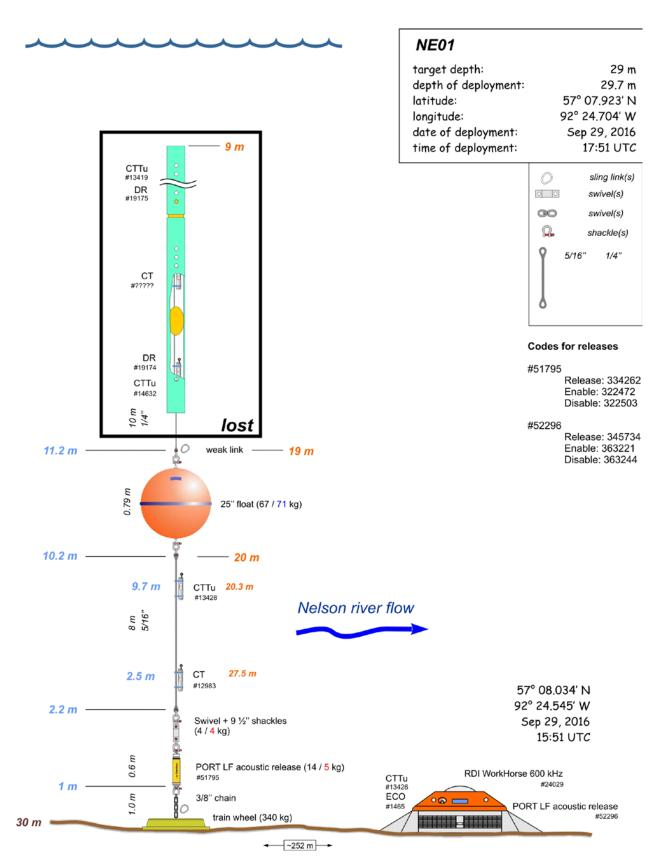
Figure 9.5 NE01 (Nelson Inner Estuary) mooring configuration, location and depth. Top tube was lost during helicopter transit.
