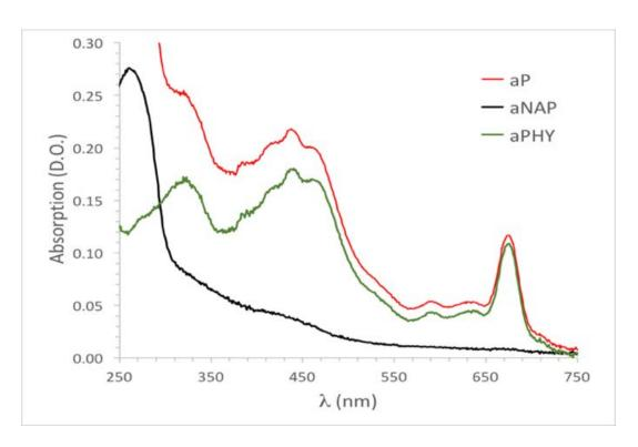
Figure 23.1. Example of spectrophotometric measu-rements of aP, aNAP and aPHY showing the relative contributions of phytoplankton and detritus to total absorption at different wavelengths.
