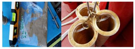
Figure 9.27 Industrial centrifuge set up, suspended sediment samples, and collection tubes
