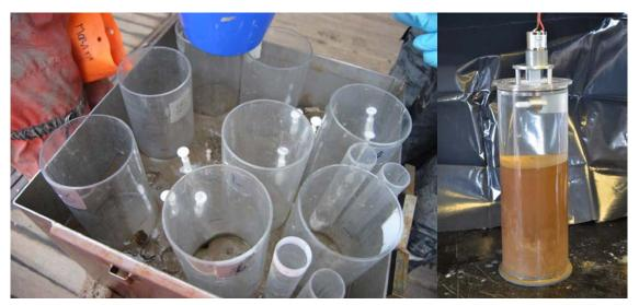
Figure 31.1. Left: Boxcore sampling, Right: Sediment core incubation set
