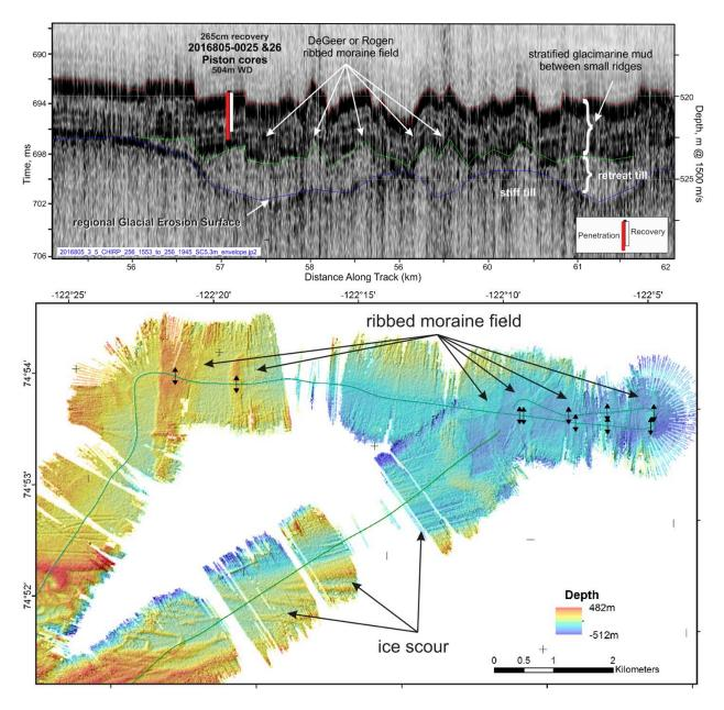
Figure 35.5. Setting of piston core Lakeman-08 (GSC stns. 20168050025 to 27) situated in the central basin of M'Clure Strait in the only known deglacial sediments not disturbed by iceberg scouring.
