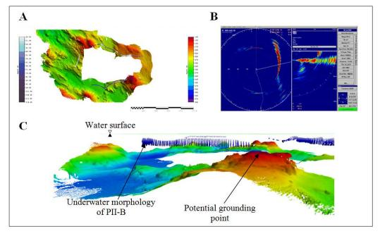
Figure 33.10. A) Seabed morphology (rainbow colorscale) around the ice island (blue colorscale represent keel depth); B) SX90 survey around the ice island. The right image shows the potential grounding site; C) Oblique 3D view of the ice island near the potential grounding area.
