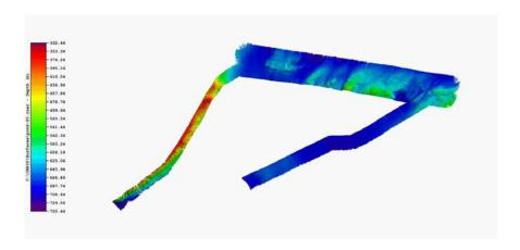
Figure 33.12. Bathymetric coverage of Pond Inlet trough survey showing glacial lineations.
