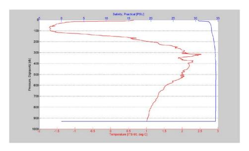
Figure 38.28 Temperature and salinity plot for rosette station 018 (ROV site 7, dive 55)
