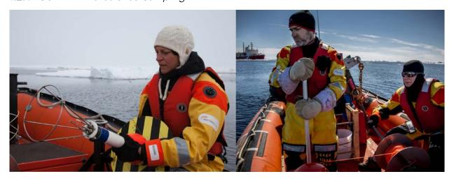
Figure 4.1. The SCAMP (left panel) and its deployment conducted from the Zodiac (right panel).
