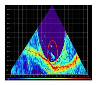
Figure 33.32. SIS water Column display of Mooring site WF1-16 after deployment. The red circle shows the buoys.
