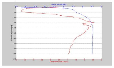
Figure 38.23 Temperature and salinity plot for rosette station 017 (ROV site 7, dive 54)
