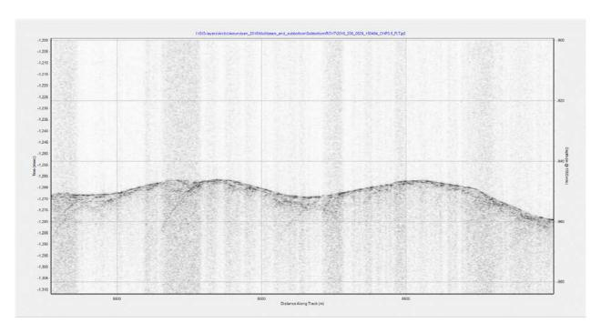
Figure 38.21 Close-up of subbottom profile at site ROV7, showing the profiles of the small ridges targeted by the piston cores. Two piston cores were collected from ridge A (2016804-014, 2016804-015), and one piston core (2016804-016) from ridge B.
