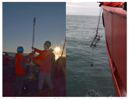
Figure 9.15 Measurements of incident solar radiation (left, radiometer attached to a stick pointing upward), total underwater irradiance and hyperspectral absorption and transmission within the water column (right, radiometers mounted to a metal frame and lowered with a weight a straight alignment)
