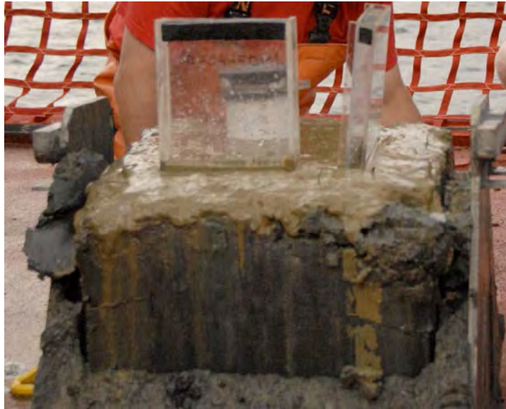
Figure 23.1. Boxcore from Anaktalak Fjord (Leg 1), with X-radiographic and pushcore subsamplers inserted, and box removed.
