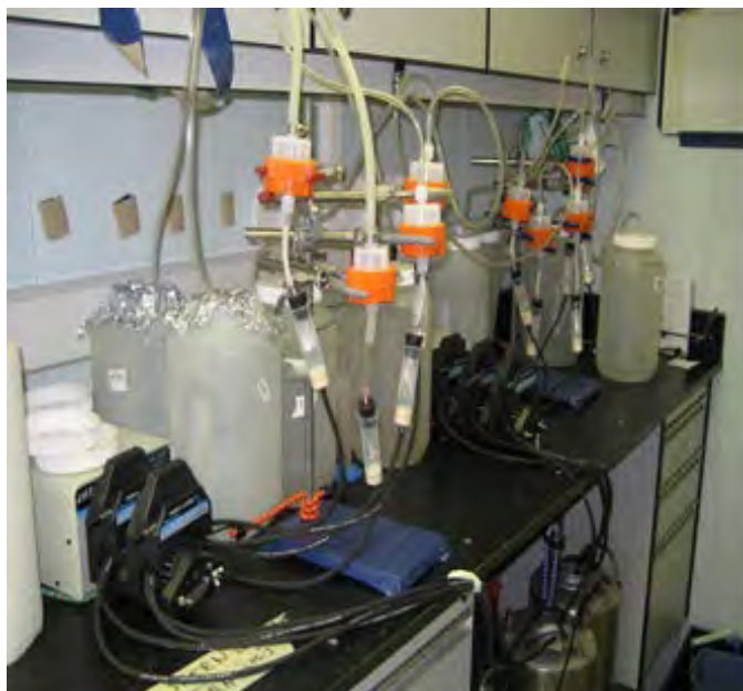
Figure 19.1. HCH water filtration in the aft chemistry lab.
