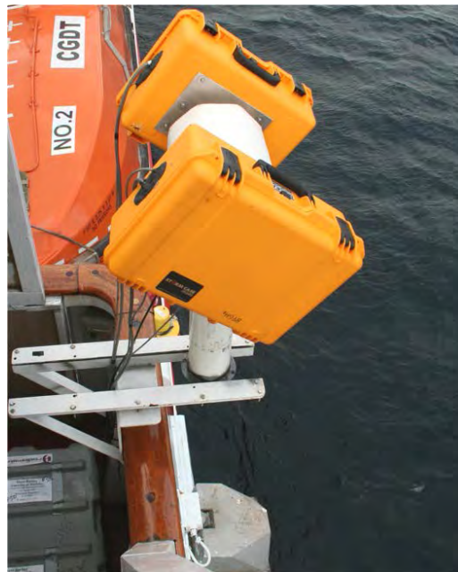
Figure 9.1. Passive microwave system, 89 and 37 GHz, installed and tested during Leg 1.
