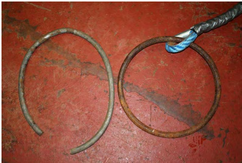
Figure 5.8. 2007 ArcticNet Beaufort Sea CA04-06 mooring salvage. Photo shows the mooring's ice-damaged acoustic release ring.
