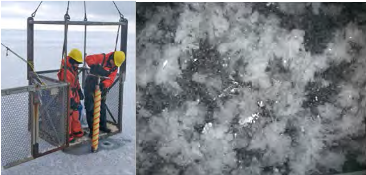
Figure 4.1. Ice cage (left) used in Ice Raids to obtain the physical-microstructure properties of snow and sea ice, and a photo of frost flowers (right) taken during an Ice Raid on 6 November.
