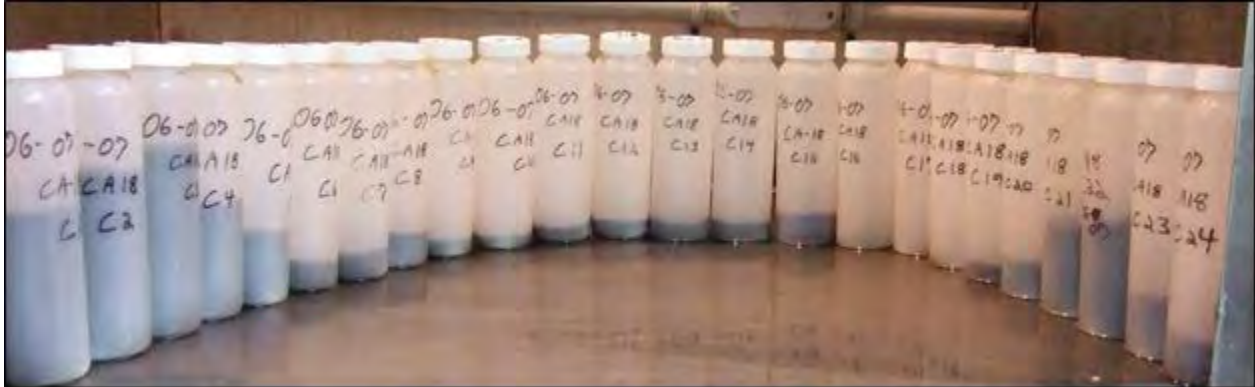
Figure 18.2. The single sediment trap time-series retrieved during Leg 3 (from CA-18, 490 m).
