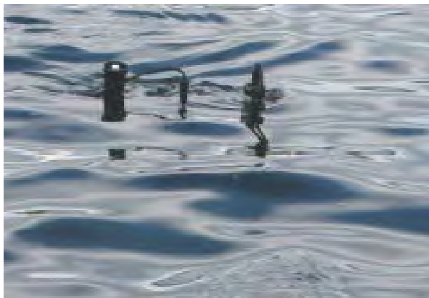
Figure 9.2. HyperOCR, hyperspectral profiling instrument at the surface.
