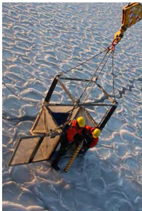
Figure 19.5. Ice cage/ice corer used to sample ice in Leg 3.
