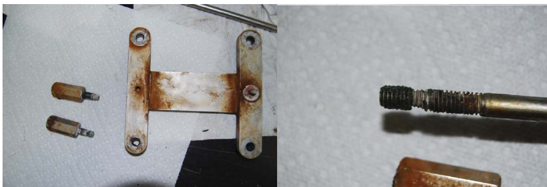
Figure 5.15. Corrosion of the CART tandem frame components (left) and tension rod thread (right) from Mooring B-09 recovered in the Beaufort Sea during Leg 2b.
