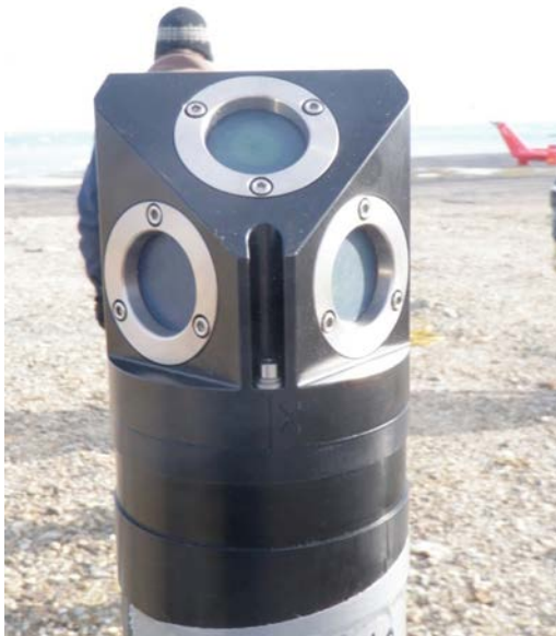
Figure 5.7. Aquadopp instrument head with indicating mark for instrument's zero heading, Lancaster Sound, Devon Island.
