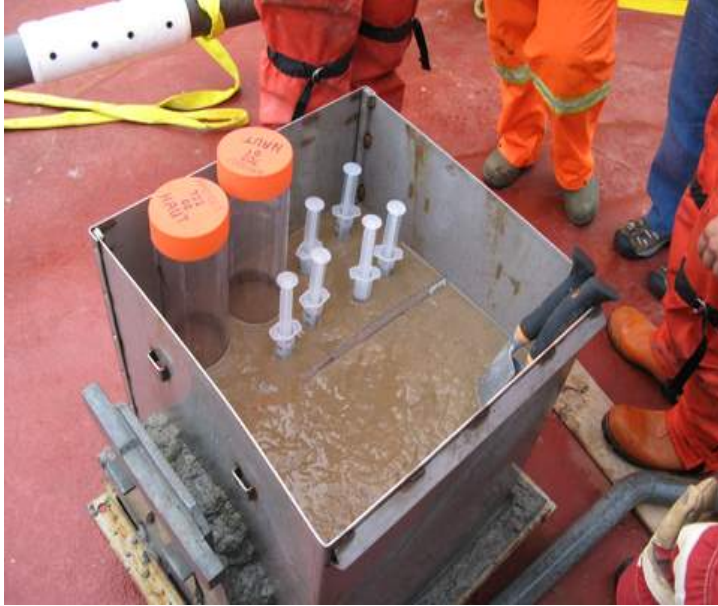
Figure 24.2. Box core with lower half for diversity/abundance sieving and upper half for OC/OM cores, pigment concentration cores and particle size grain cores (white syringes).
