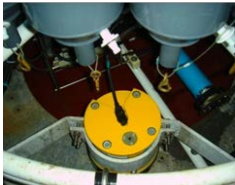
Figure 6.2. LADCP equipped on the Rosette frame during Leg 2 to measure currents in the water column.
