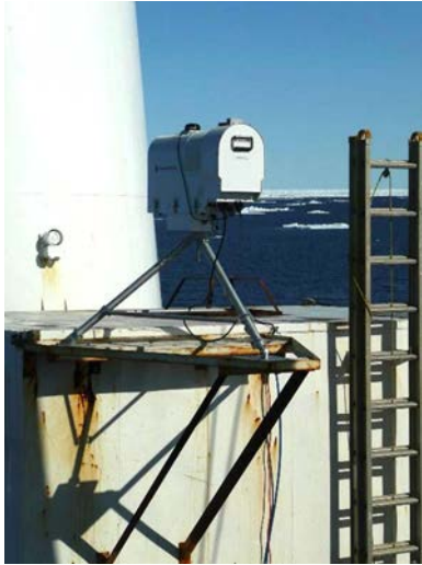
Figure 3.9. The temperature and water vapour profiling radiometer (TP/WVP 3000A) mounted on the roof of the MetOcean Container.
