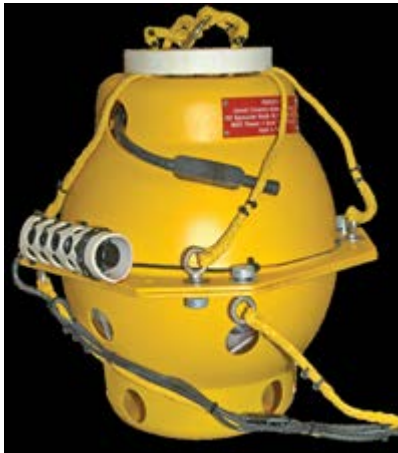
Figure 15.1. Marine Autonomous Recording Unit deployed in the Beaufort Sea during Leg 2a.
