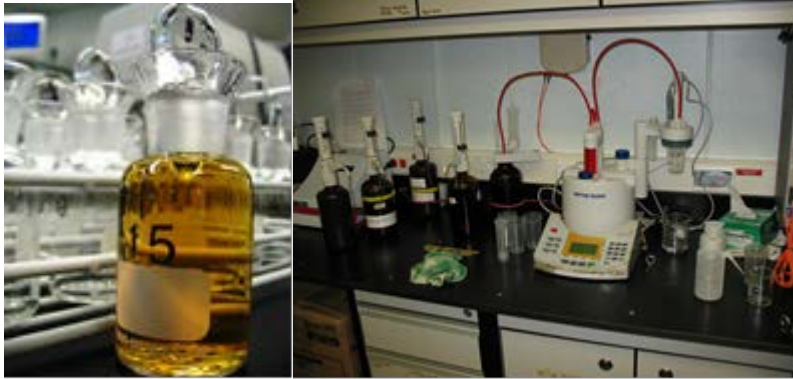
Figure 6.5. Bottles used to collect samples (left) for oxygen calibration and the Mettler Toledo titrator (right) used to analyze the samples onboard the Amundsen .
