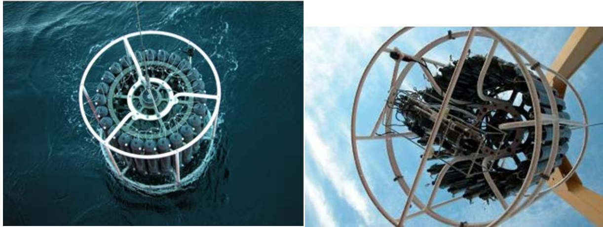
Figure 6.1. CTD-Rosette system used on the Amundsen to characterize water column properties and collect seawater samples. Photo on the right shows the different sensors located below the bottles
