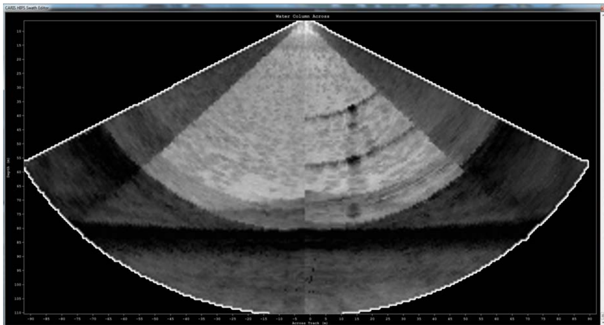
Figure 5.18. Multibeam water column imagery identifying orientation and instrument depths for deployed moorings (Screenshot courtesy of ArcticNet multibeam processing team).
