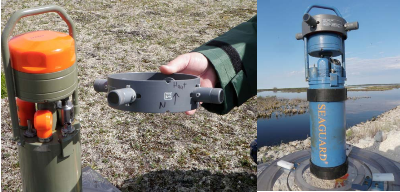
Figure 5.10. Left: Reading stabilizer for Aanderaa instruments. Right; RCM-Seaguard #30 with water current simulator affixed. Photos from ADCP compass calibration site in Churchill River (causeway), Hudson Bay, on 20 July 2010: 74° 34.3367' N, 80° 43.7241' W – Mag. Decl. 2°.
