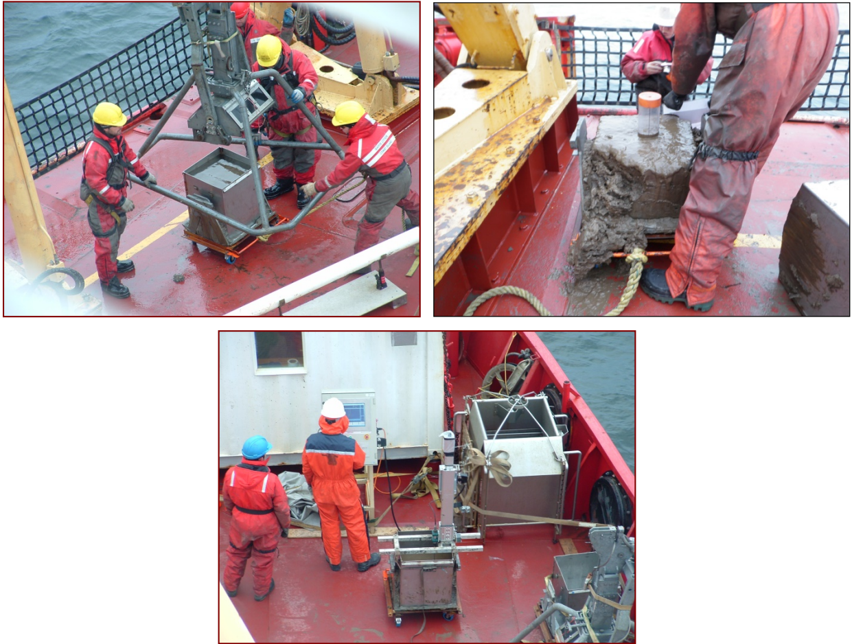
Figure 22.7. Box core deployment and sub-sampling (Photos: C. Breton and J.Buis).
