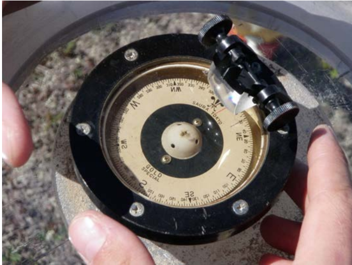
Figure 5.6. Analog compass used for magnetic declination verification during the compass calibrations in the field.
