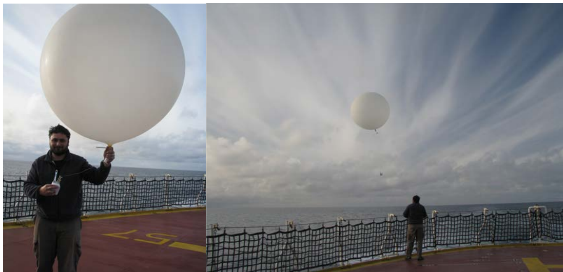
Figure 3.10. A weather balloon with attached radiosonde and the launch from the helicopter deck (Photos: M. Gervais).
