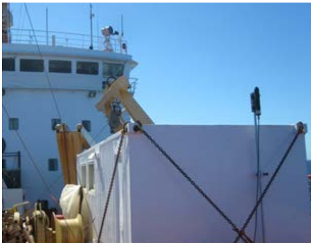
Figure 8.3. HyperSAS sky irradiance sensor used during Leg 1a.
