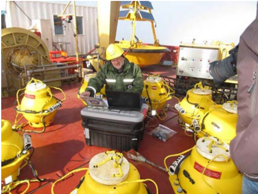
Figure 15.2. Synchronizing the MARUs on the deck of the Amundsen before deployment on 15 August 2010 in Leg 2a.
