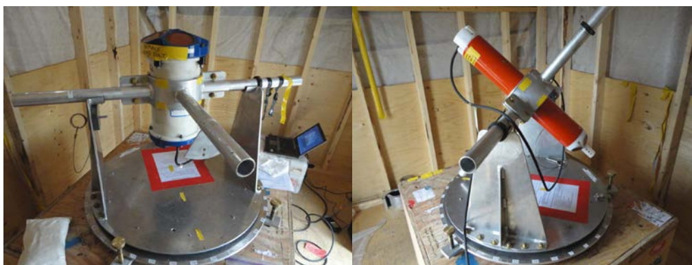
Figure 5.9. Mooring instrument compass calibration performed in Inuvik, NWT using a jig with a RDI WHS (left) and a RDI DVS750 (right) (Golder Cruise Report Leg 2, 2010).
