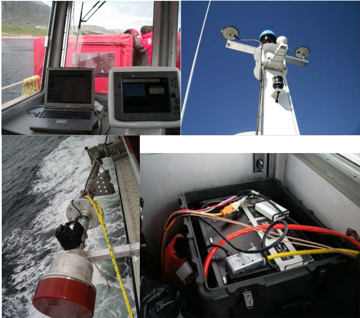
Figure 20.2. Barge setup to conduct multibeam mapping surveys: EM302 operator station (upper left), Positioning and motion antennas (upper right), Pole mount with multibeam and surface sound speed probe (bottom left) and Server rack (bottom right).
