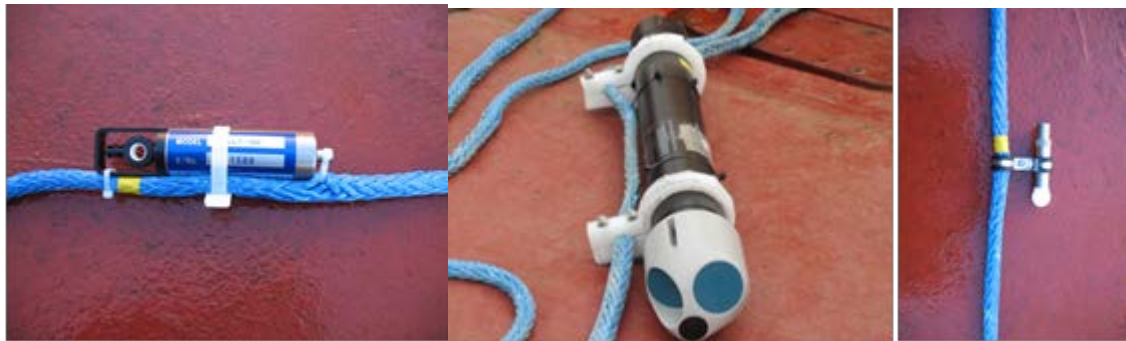
Figure 3.6. [Left] JFE ALEC ® compact CT sensor. [Middle] Aquadopp current profiler. [Right] JFE ALEC ® PAR sensor (Photo: E. Stainton).
