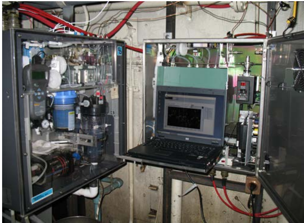
Figure 2.4. The on-track pCO 2 system located in the engine room of the CCGS Amundsen . The equilibration chamber is the clear cylinder (left, vertical with black top) and the gas analyzer is the green box behind the computer display.
