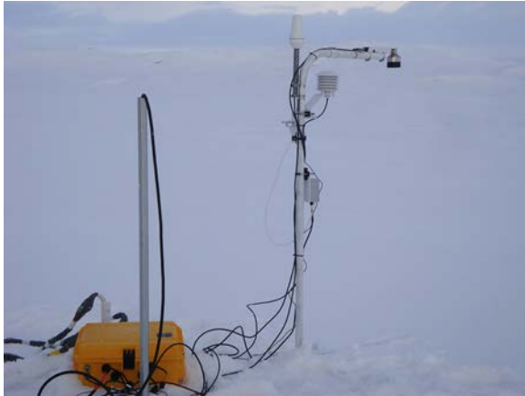
Figure 3.5. Ice mass balance system (CEOS IMB04) installed in the Beaufort Sea on 27 September 2010 during Leg 3a.
