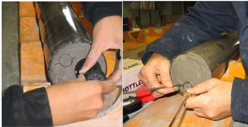
Figure 22.6. Left: Taking a Torvane measurement on one of the cores. Right: Inserting a constant volume sampler. (Photos: K. Jarrett)
