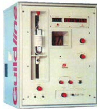
Figure 6.3. Bottles used to collect samples (left) for salinity calibration and the Guildline instrument (right) used to analyze salinity samples onboard the Amundsen .
