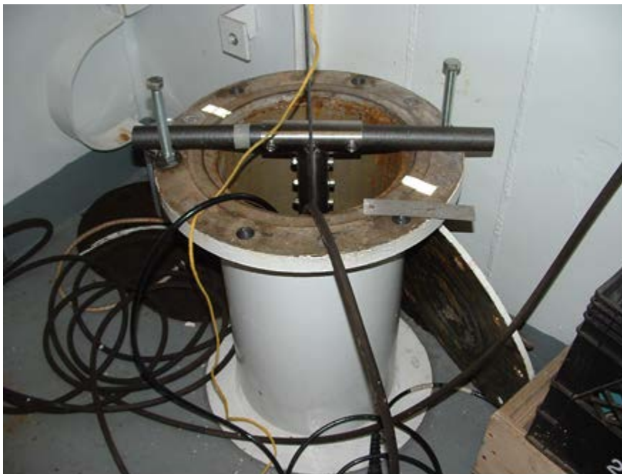
Figure 22.4. USBL transducer deployed in the acoustic well.
