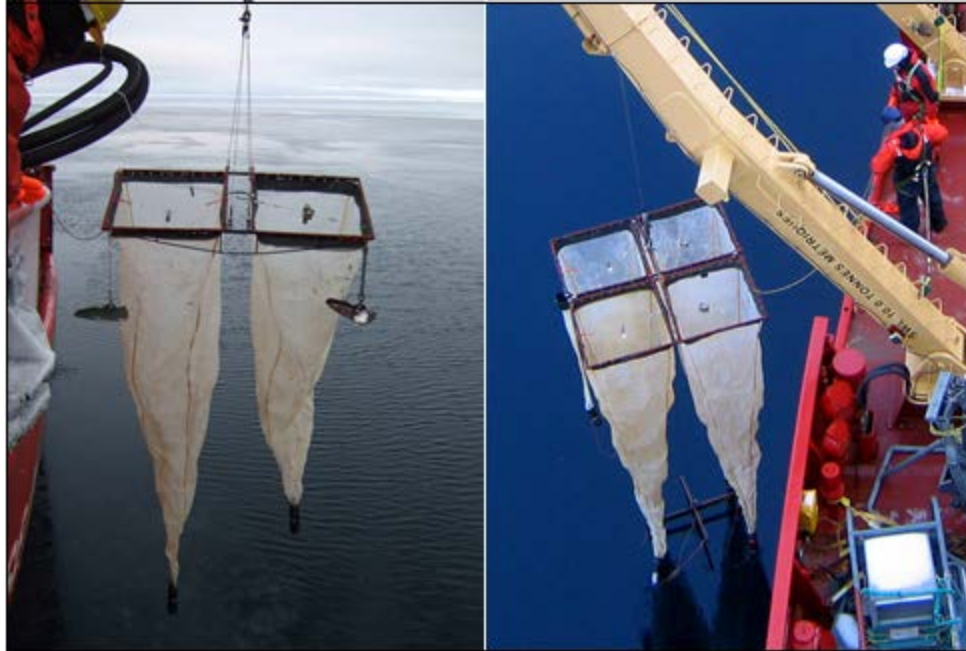
Figure 13.1. Zooplankton and fish sampling gear used during Leg 1. Left: 2 x 1-m 2 Tucker net and Right: 4 x 1-m 2 Monster net. (Photos were taken during previous ArcticNet expeditions).
