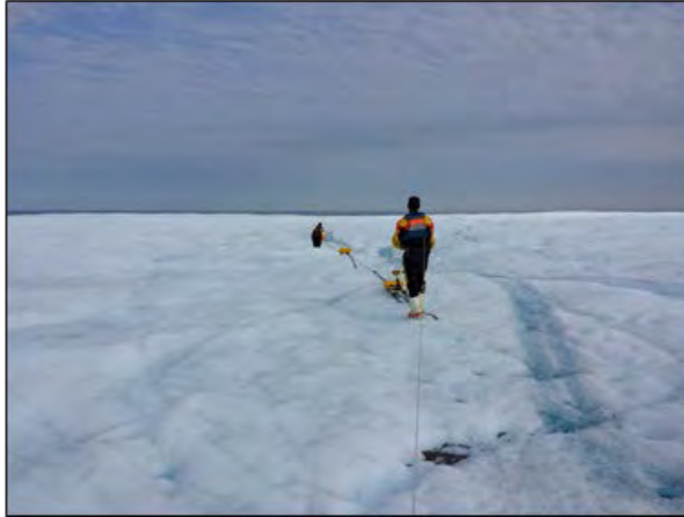
Figure 5.2. The GPR system being towed during the 500 m transect.
