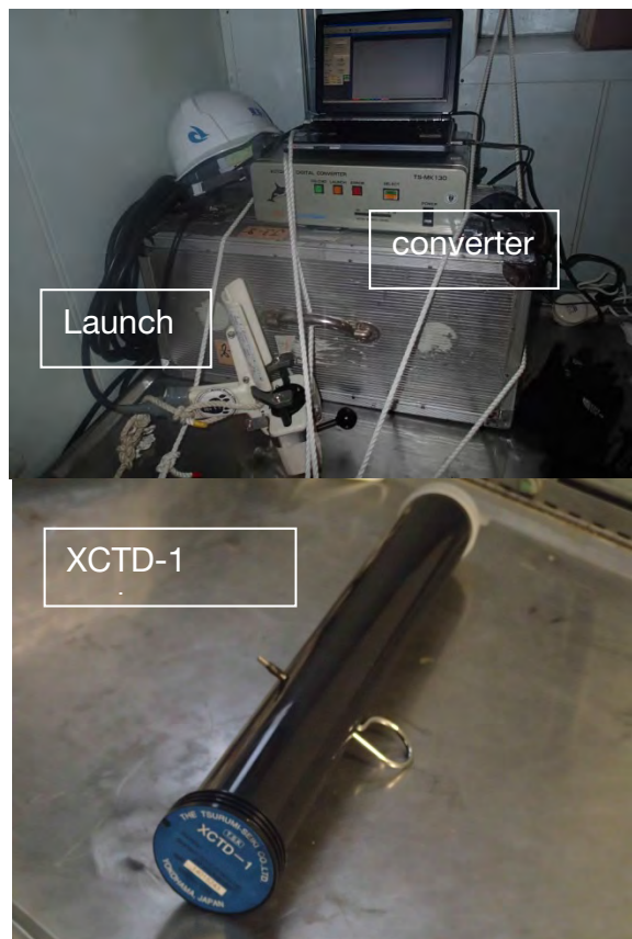
Figure 12.1. The XCTD system at the after deck. (Upper) the digital converter MK-130, the launcher and a PC for operation, (Lower) a XCTD-1 probe. XCTD-1 probe can measure temperature and conductivity from ocean surface to 1100 m water depth. Depth (m) is calculated from the time started from when a XCTD probe enters the ocean.
