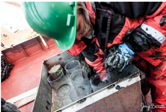
Figure 20.3. Push coring the boxcore (photo: Jessy Barrette 2013 ArcticNet Leg 1a).
