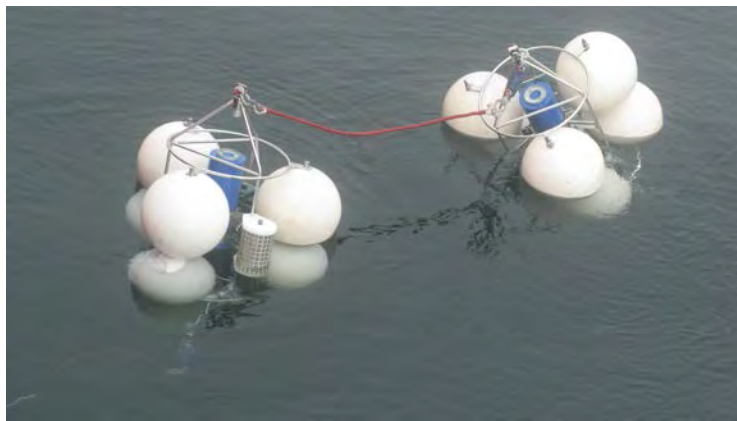
Figure 20.4. SPMD cage installed on ArcticNet mooring BS-3.
