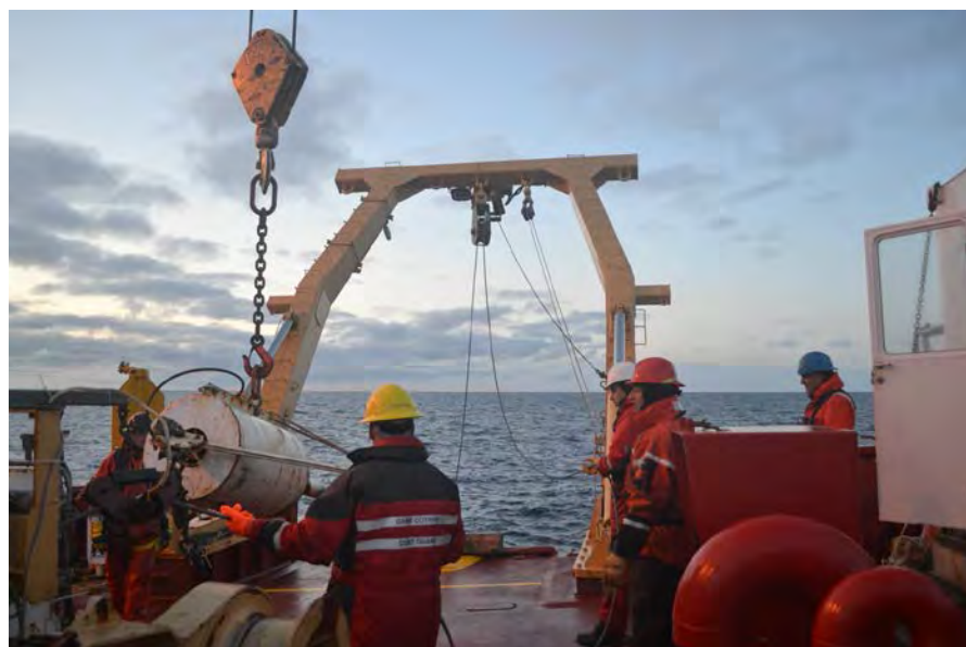
Figure 29.1. Deployment of the piston core.
