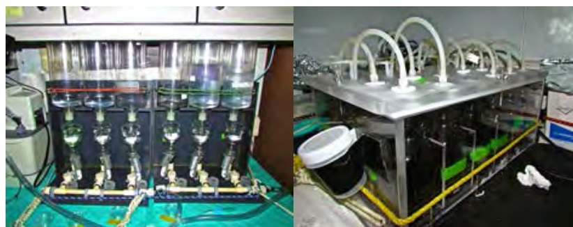
Figure 10.3. Filtration systems used for: Absorption of particulates (left), and absorption of colored dissolved matter (right).
