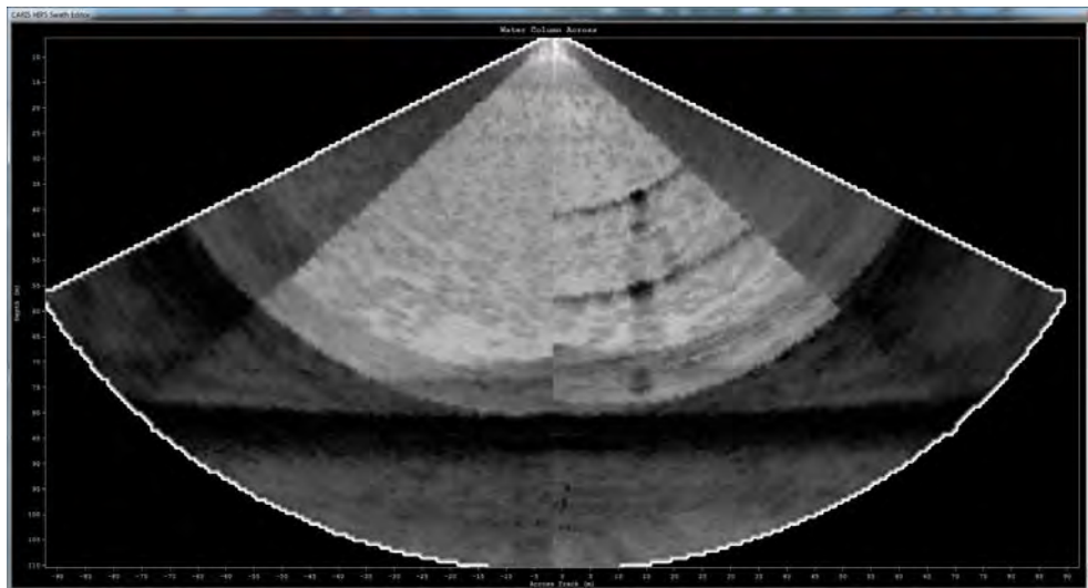
Figure 7.13. Multibeam imagery identifying orientation and instrument depths (screenshot courtesy of ArcticNet multibeam processing team).
