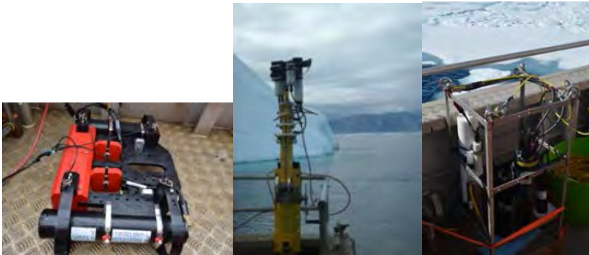
Figure 10.2. Instruments measuring water column parameters: Radiometer (left), Reference radiometer, GPS and Bioshade used on the barge (centre), and Optical instruments (right).
