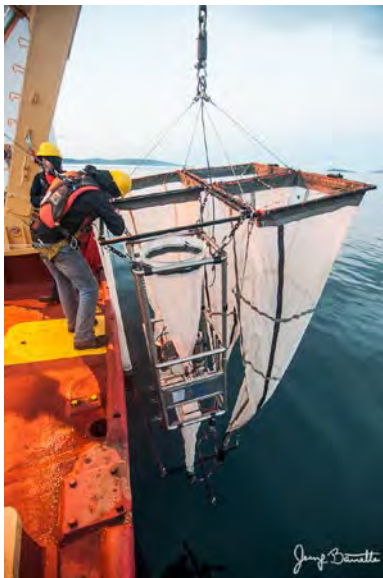
Figure 20.1. The 5-net vertical zooplankton sampler with LOKI (Monster net).
