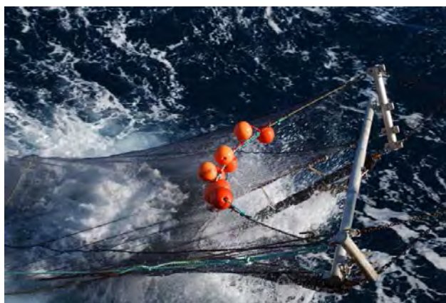
Figure 19.1. The beam trawl being retrieved. Photo credit: Gordon Chamberlain.
