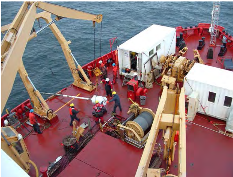
Figure 30.1. Piston corer being retrieved on CCGS Amundsen .
