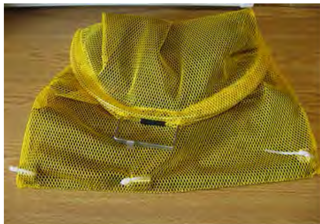
Figure 27.2. Sample bag used for sampling by the ROV. Weights were used to keep the bag straight in the water.
