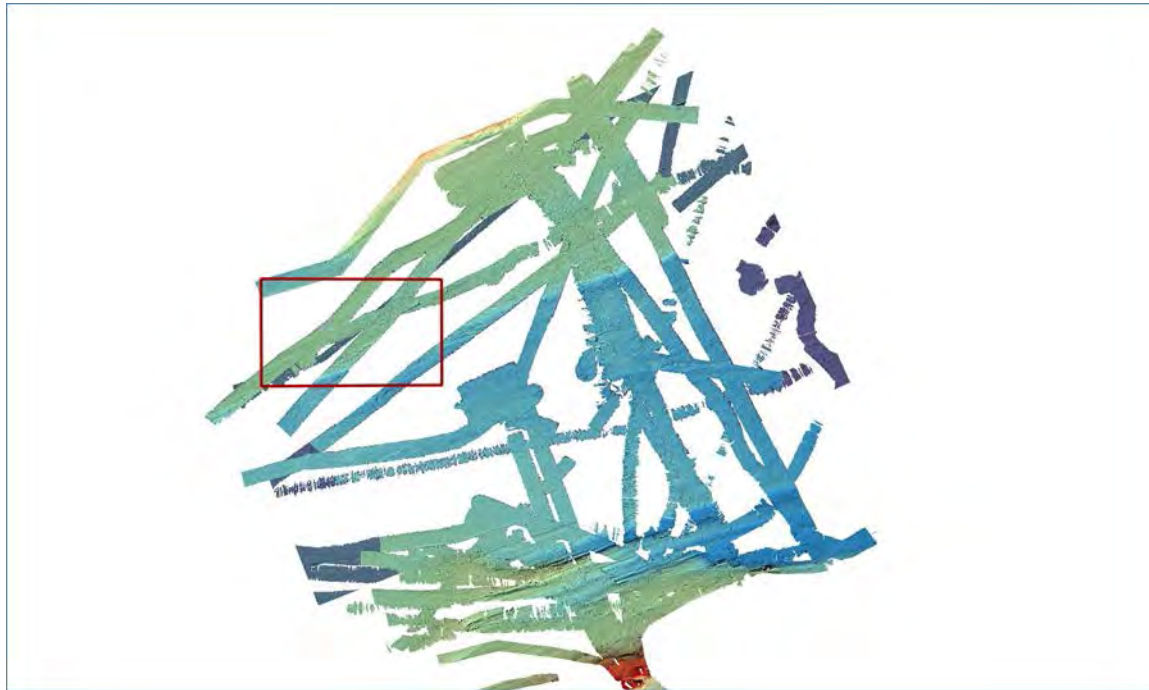
Figure 23.2. Grid of the 2003 to 2014 EM302/EM3002 bathymetry coverage for the eastern portion of Lancaster Sound. The UNB basemaps are still visible underneath due to the limited extent of the generated grid. The area within the polygon is depicted in Figure 23.3.
