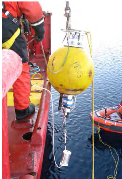
Figure 20.5. SPMD cage installed on the line on BREA mooring BR-3.
