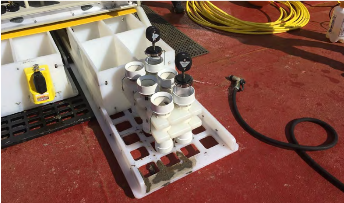
Figure 5-5: Positioning of push-cores on extensible tray during the 2020 ROV trials. Two additional push-cores could potentially be added to the frame, which would extend to the red polygon area.
