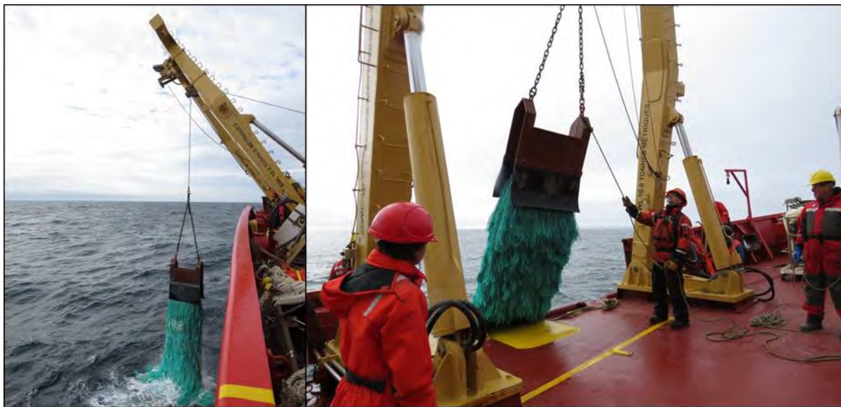
Figure 2-3: Rock dredge deployment in 2019. The same equipment was used in 2020
