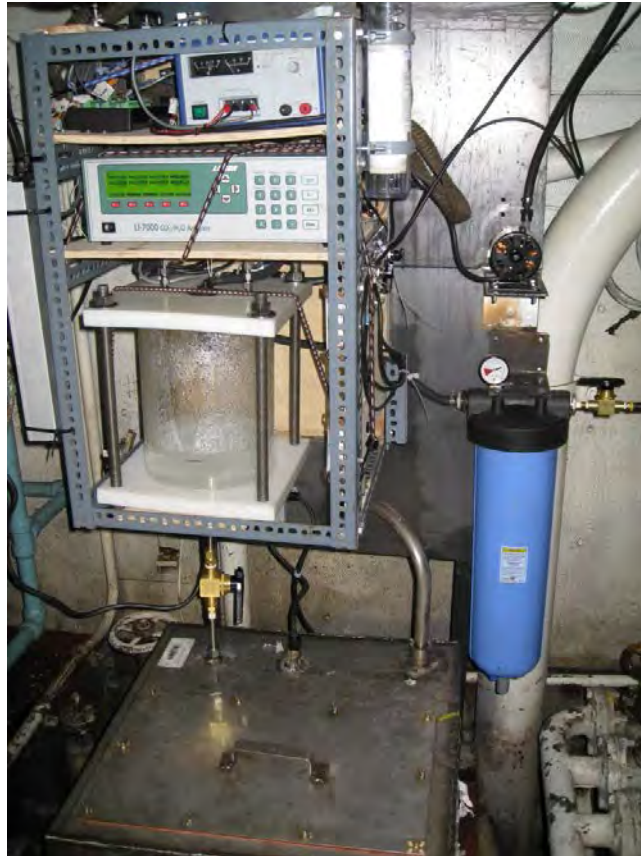
Figure 2.2. The on-track pCO 2 system located in the engine room of the Amundsen . The equilibration chamber is the clear cylinder (left bottom) and the gas analyzer is the box with the digital display.
