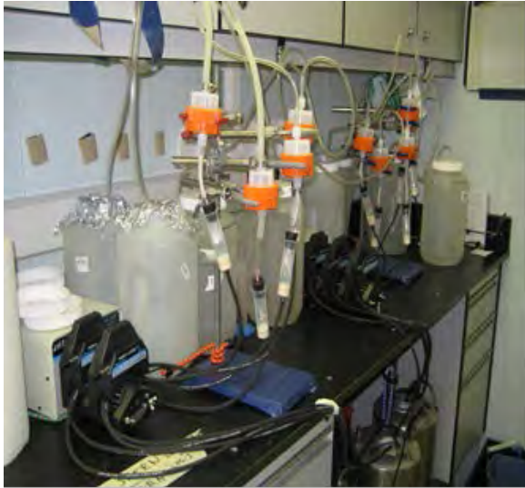
Figure 14.1. HCH water filtration in the aft chemistry lab.
