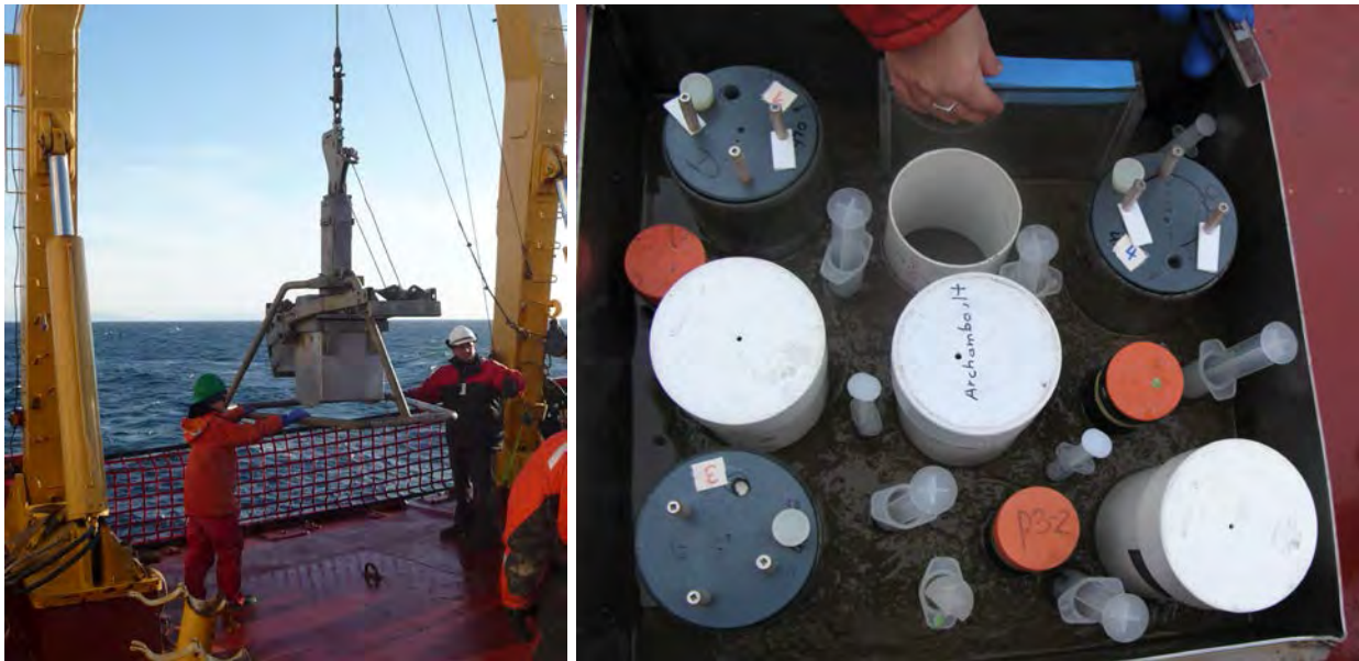
Figure 17.1. Left : The box corer is being deployed. Right : Box core with SOD/Nutrient cores (grey), bioturbation cores (white), pigment concentration cores (orange), CN cores (big syringes), Meiofauna samples (big syringes), Meiofauna/Microfauna incubation samples (small syringes), and X-ray tray and push core for Sam Bentley.
