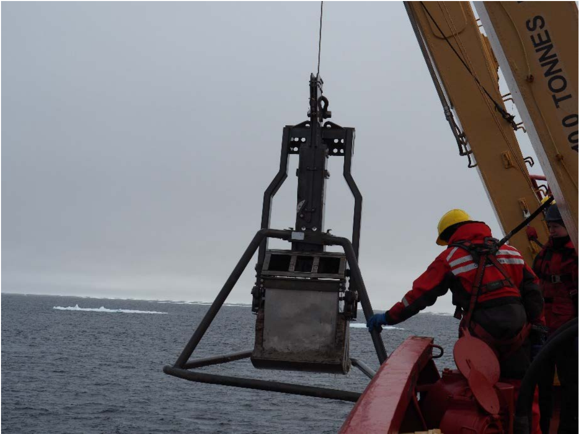
Figure 29.1 Recovery of full box core
