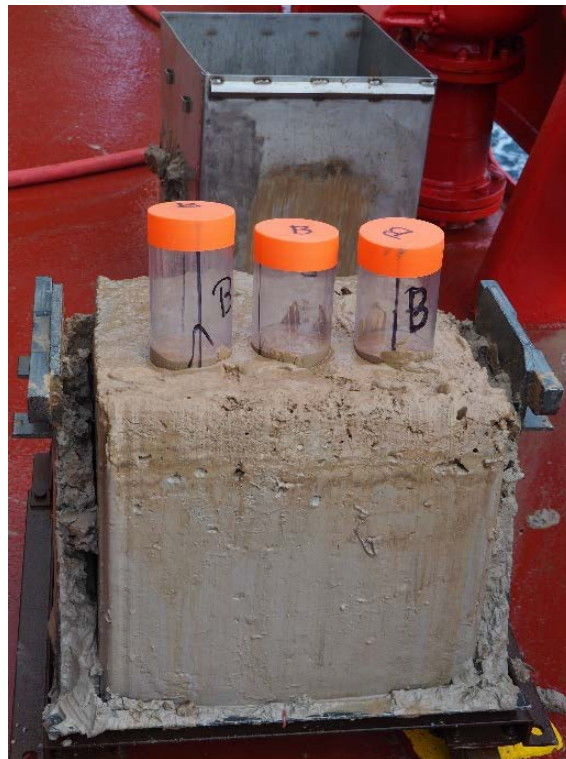
Figure 29.2 Push cores in open box core, prior to extraction
