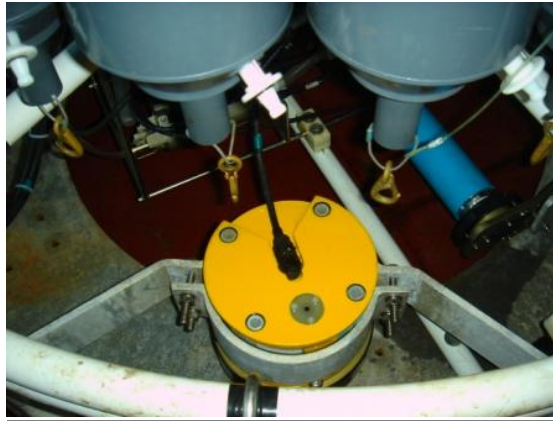
Figure 7.4 Lowered Acoustic Doppler Current Profiler (LADCP)
