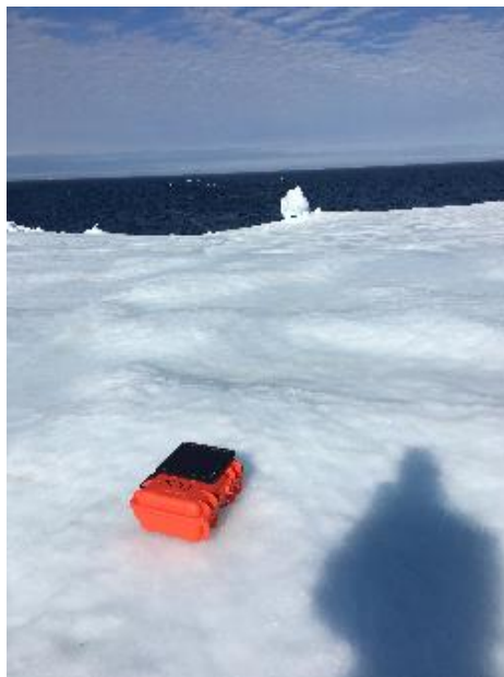
Figure 4.3 Example of placement of beacon on iceberg. Deployed E of Manson icefield July 25, 2017. Photo: Abby Dalton.
