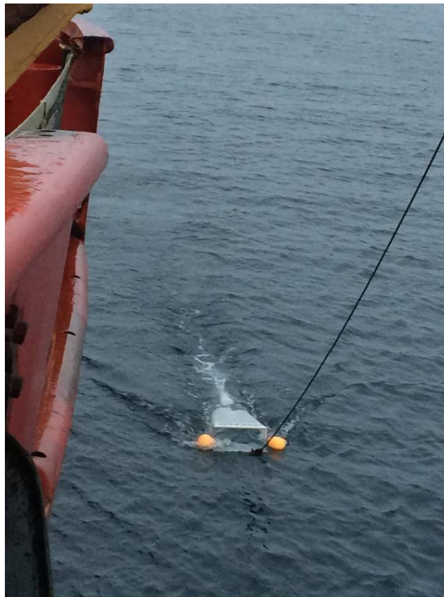
Figure 18.3 Manta Net Deployment
