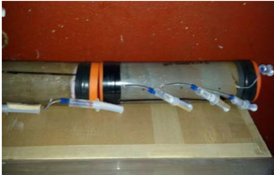
Figure 29.5 Push (up) and gravity (down) cores drills and undergoing subsampling for pore water using rhizons. Push core is approximately 50 cm long
