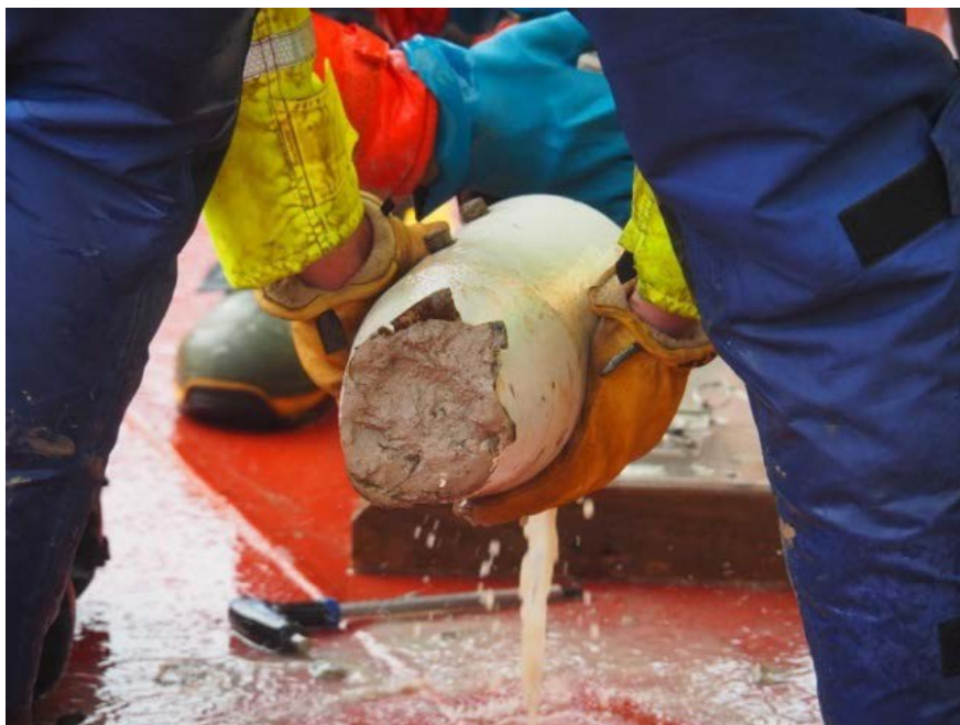
Figure 29.7 Damaged piston core cutter being removed from the lowermost core barrel. Note splayed and deformed cutting edge
