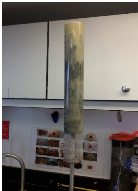
Figure 29.3 Extruding small push core for geochemical analyses
