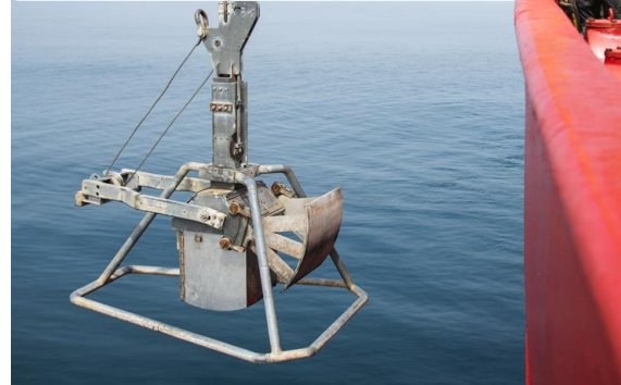
A box corer is a marine geological sampling tool for minimum disturbance of soft sediments.
