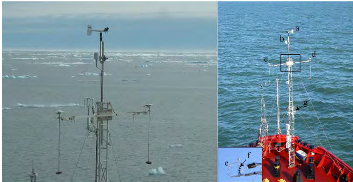
Figure 4.2. Upper section of the tower showing: (a) wind monitor; (b) shielded temperature-relative humidity probe; and gimbaled (c) pyranometer and (d) pyrgeometer; (e) sonic anemometer; (f) open-path CO 2 /H 2 O sensor. (g) The motion sensor is located outside of the picture.
