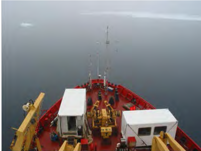
Figure 4.1. The foredeck of the CCGS Amundsen equipped with a meteorological tower for surface meteorology and CO 2 flux measurements.
