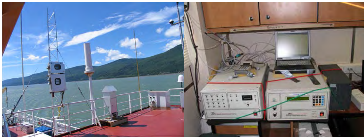
Figure 3.2. Left: Mercury speciation units (Tekran) (left) and Hi-Vol Organic sampler (PS-1) (right). Right: Pump module and Tekran analyser for Hg speciation in the acquisition room.
