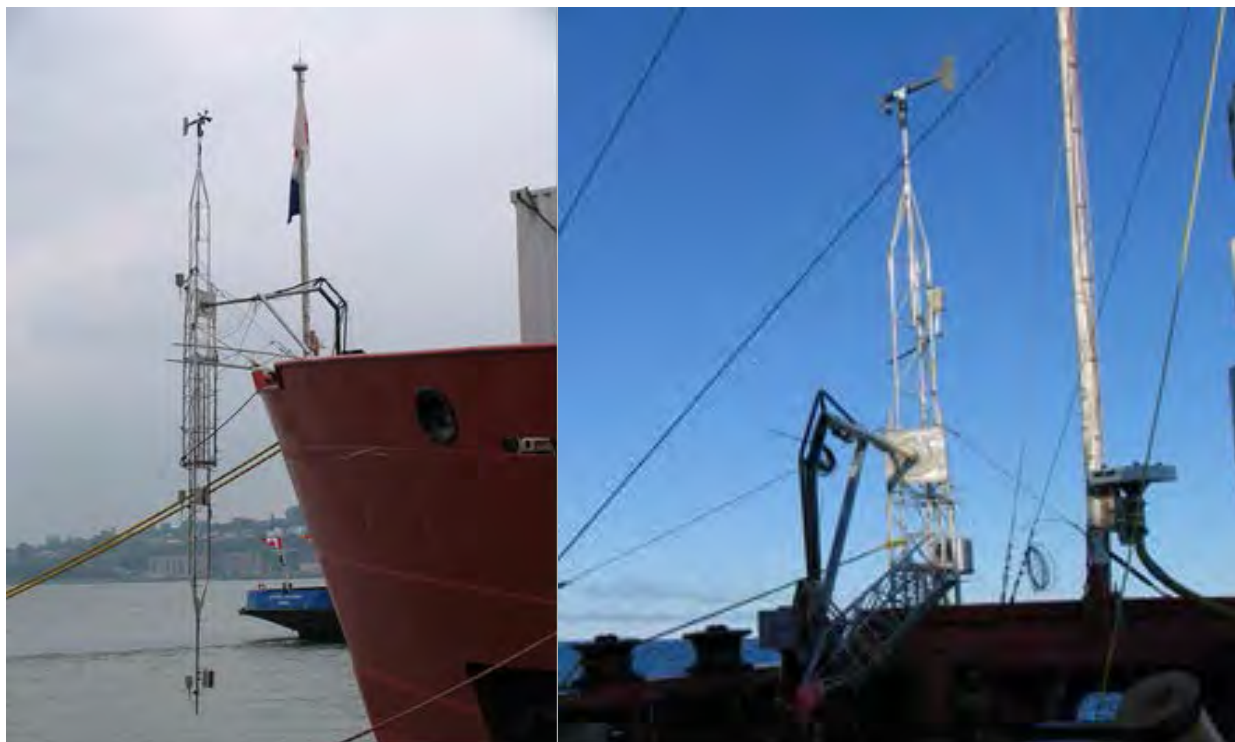
Figure 3.1. Left: Gradient tower profiler at the bow of the ship. This setup permitted air sampling at two heights ( \Delta \sim 2 m) and air temperature gradient measurements at three heights (2, 4 & 6 m) within the marine boundary layer. Wind direction and wind speed as well as solar radiation were monitored in continuous mode. Right: securing set-up for the tower.
