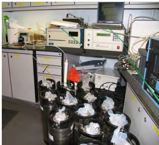
Figure 3.4. Herbicides sampling set-up, canisters and pump.
