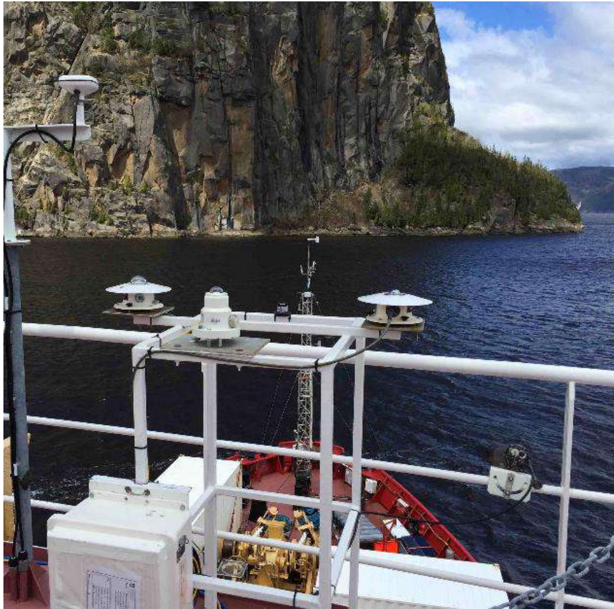
Figure 1-1 The radiation sensors and digital camera located above the wheelhouse of the Amundsen. Shown are the pyrometer (right), pyranometer (left) and PAR sensor (centre back) and UV sensor (centre front). The automated digital camera is mounted on the rail below and to the right of the pyrometer.
