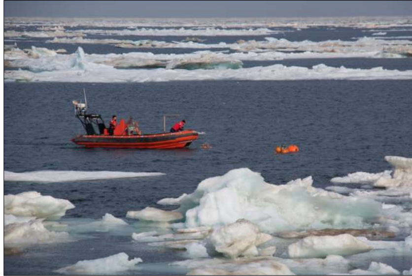
Figure 5-2 Mooring recovery with an assistance of zodiac
