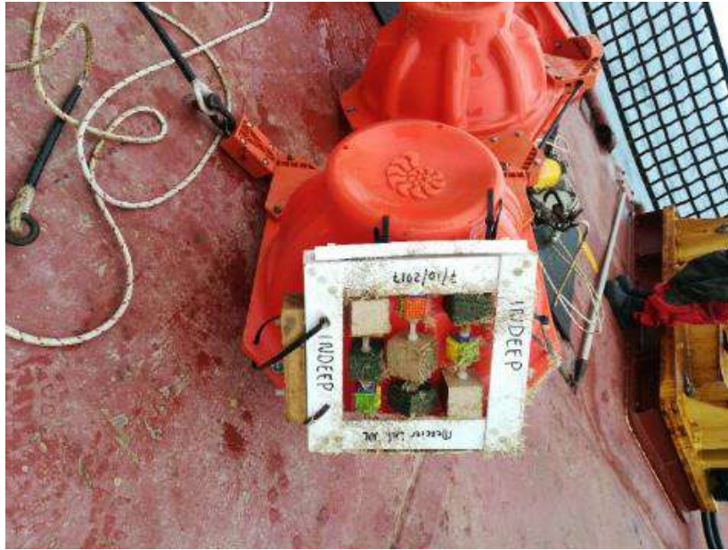
Figure 11-5 Settlement apparatus recovered from the site HiBioA-17 with colonies of hydrozoans attached.
