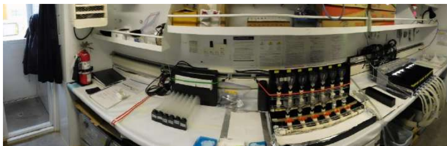
Figure 8-3 General set-up for the PE incubations in the Radvan. From right to left: inoculation space, incubator, filtration ramp, clean work space (Photo Credit: Rachel Hussherr).
