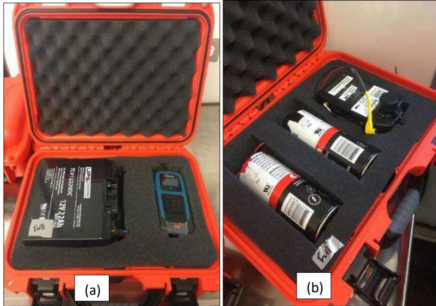
Figure 3-1 Iceberg tracking beacons: (a) Rockstar Iridium and (b) Solara Iridium Photos: Abigail Dalton.
