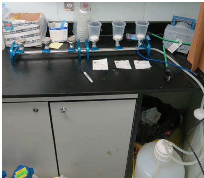
Figure 16-1 Manifold used for water filtration of water for microbiology. Water from the amber glass bottles was filtered through 0.2 \mu\text{m} inline membrane filters. The filtrates of this filtration were acidified to pH 2 using hydrochloric acid and the dissolved organic matter (DOM) was extracted with methanol using solid phase extraction (as per Dittmar et al., 2008) with a styrene-divinylbenzene polymer sorbent (Agilent Bond Elut PPL, 5 g). Methanol extracts were stored in the dark in glass vials at -20°C for future Fourier transform ion cyclotron resonance mass spectrometry (FTICR-MS) analysis to characterize the dissolved organic carbon.
