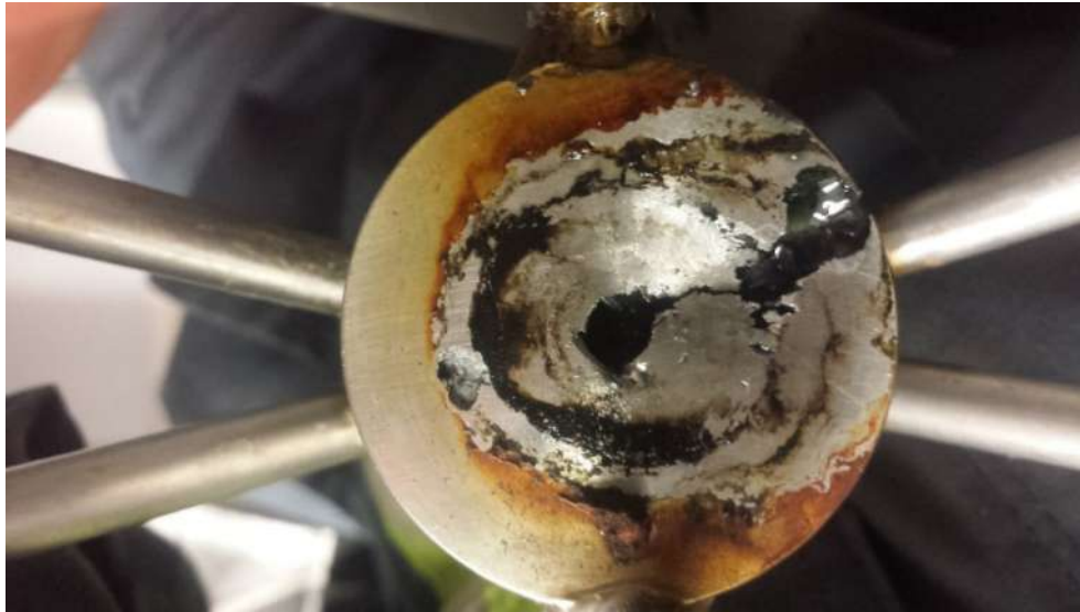
Figure 6-11 HiBioA-17 Recovered Aquadopp Profiler frame corrosion
