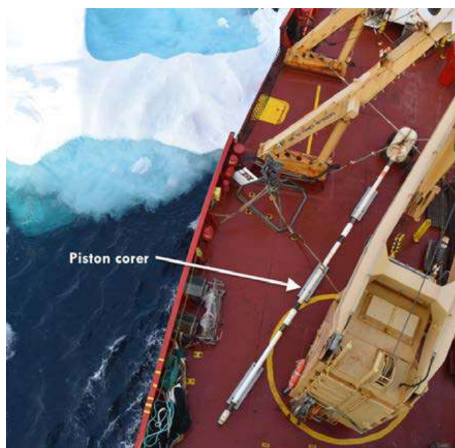
Figure 36-8 Piston corer on the fore-deck of the CCGS Amundsen awaiting connection and deployment Table 43-5 Piston coring operations: location, depth, identification, and characteristics. Core site are shown graphically in Figs. 8. PC = Piston Core; TWC = Trigger Weight Core; GC = Gravity Core; BC = Box Core (including sequentially lettered push cores from the box core); surface = surface samples from box core only.
