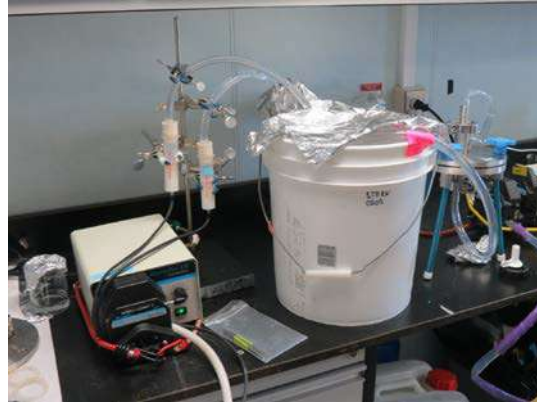
Figure 16-3 Filtering and organic matter trapping apparatus for hydrocarbon measurement
