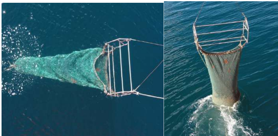
Figure 28-1 Agassiz trawl used to catch epibenthic organisms on board of the CCGS Amundsen
