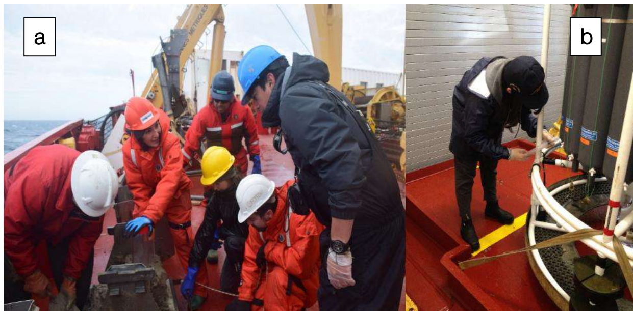
Figure 13-1 Sampling from a box core (a, © Shaomin Chen) and from CTD-Rosette (b, © Karl Purcell).
