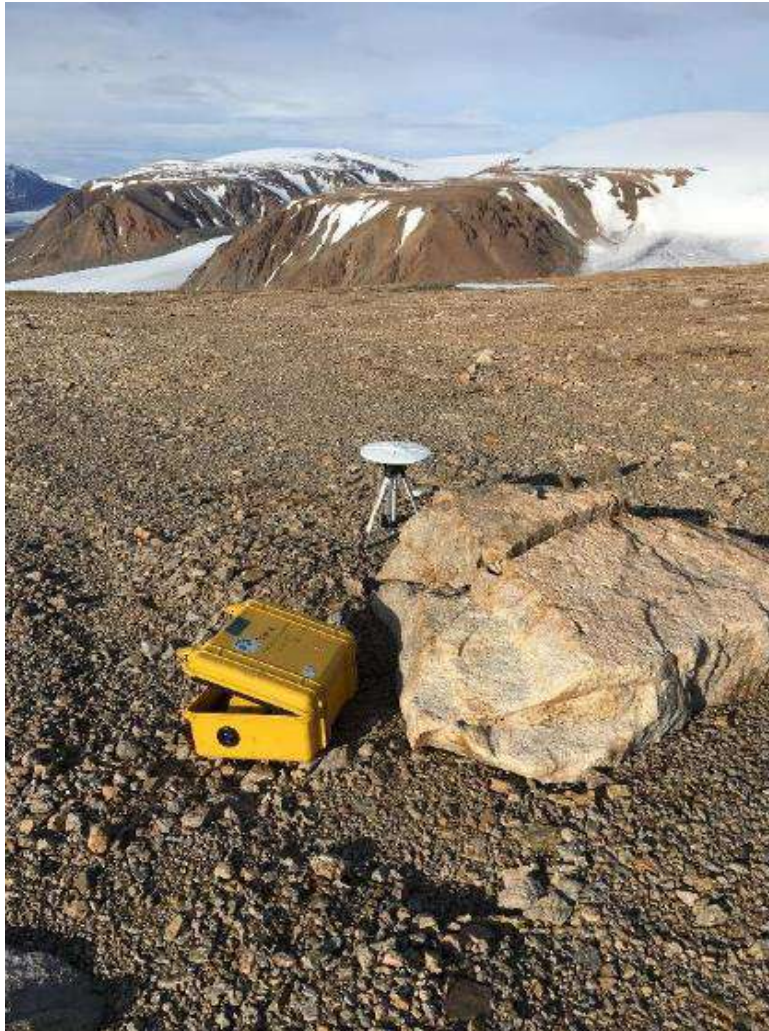
Figure 3-11 Trimble R7 GPS unit set-up near a boulder in the footprint of the Manson 2 survey (see green star in Figure X2). Photos: Claire BGM.
