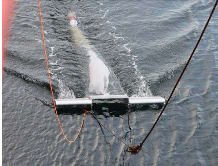
Figure 37-30 Manta trawl deployment for microplastic sampling in Frobisher Bay during Leg 2c of the 2018 CCGS Amundsen expedition.
