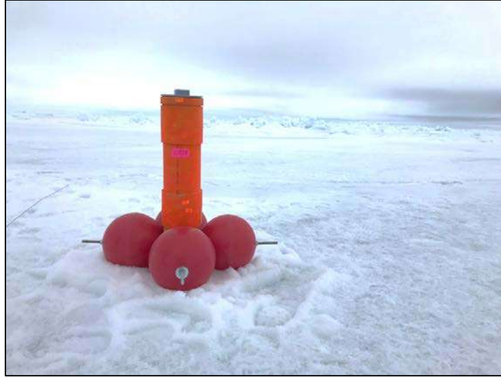
Figure 2-4 The surface portion of the ice-tethered mooring. There is a GPS tracker within the surface unit that allowed us to recover the unit after 6 days
