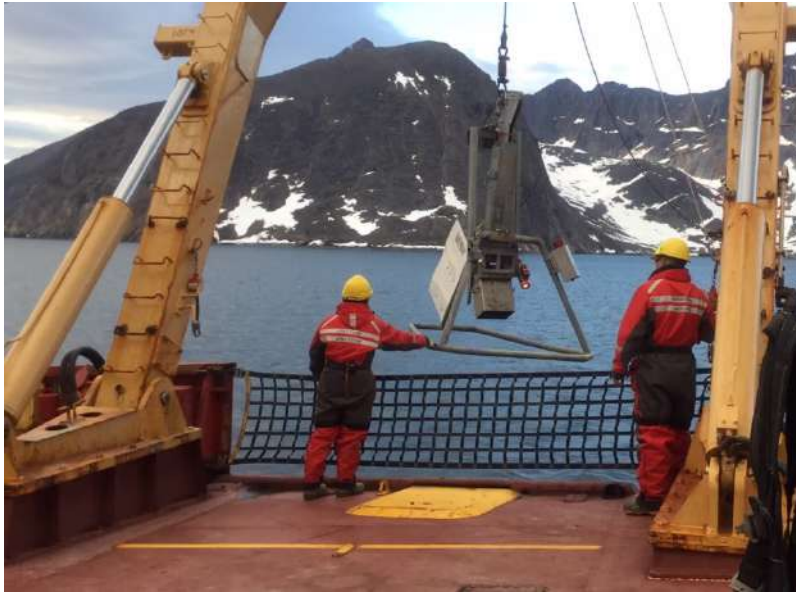
Figure 33-3 . DFO (NL) drop video camera, the “Frankenbox”, being deployed in outer Frobisher Bay. Photo © David Coté.
