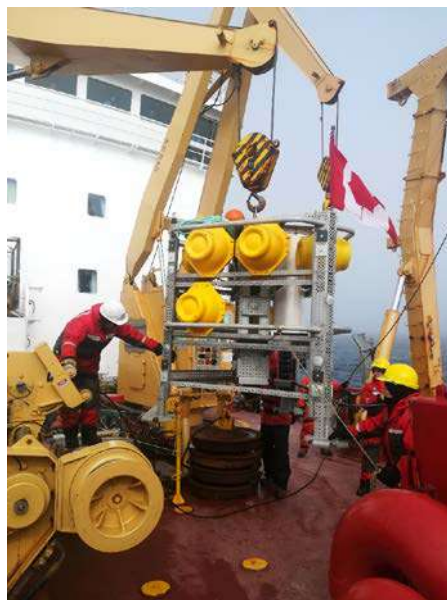
Figure 11-8 Operations during the deployment of lander and settlement apparatus attached, on July 30th, 2018.
