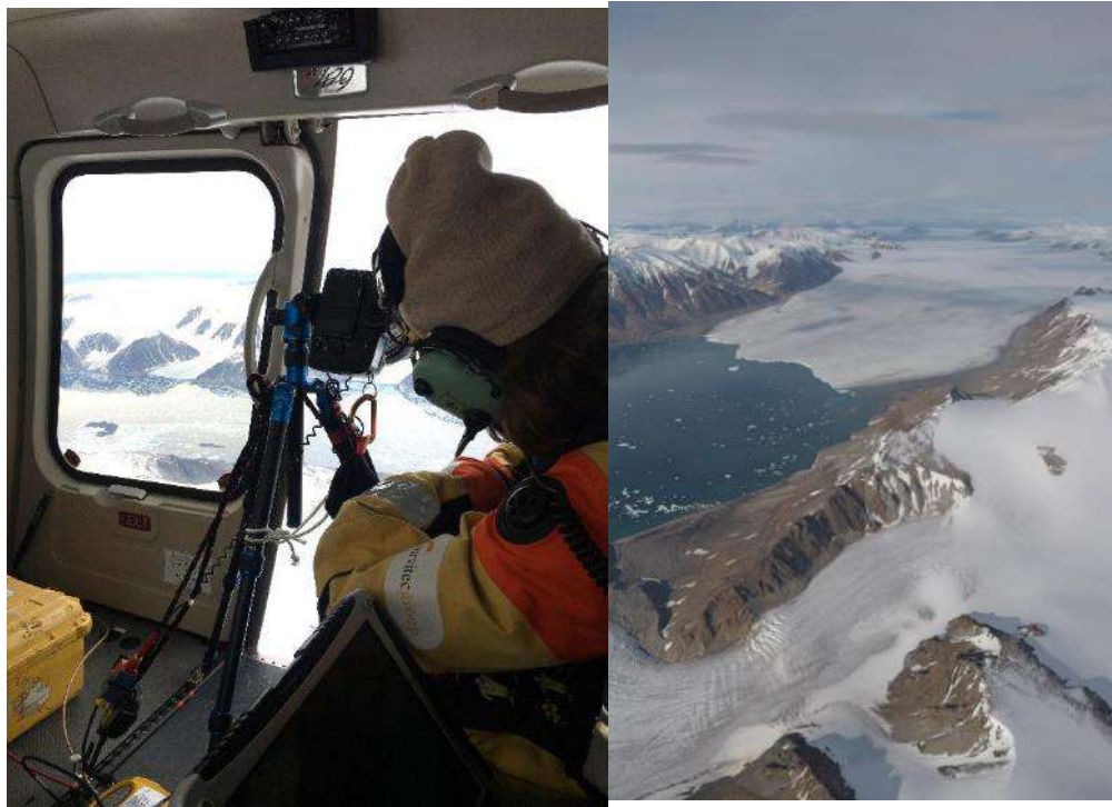
Figure 3-10 Set-up of the camera (Nikon D850) and differential GPS (Trimble R7 in yellow box) in the helicopter (left) and example of photo from Manson 2 survey that will be used to create the DEMs (right). Photos: Abigail Dalton and Claire BGM.
