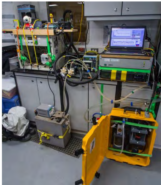
Figure 13-1 The underway gas measurement instruments in the Amundsen's paleo/geology laboratory. The MIMS is highlighted in blue, and the optode/GTD system in red. Seawater was pumped to the instruments from the seawater tap (to right of image)
