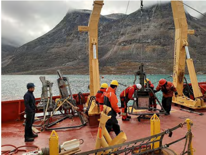
Figure 26-3 Box coring in Southwind Fjord, Baffin Island.
