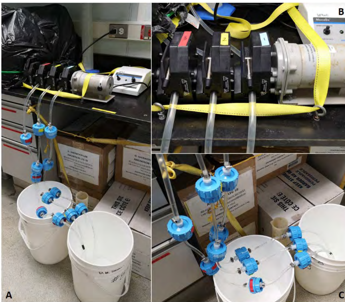
Figure 6-1 Overview of the filtration system (A). The setup of the pump for filtering 3 samples at the same time (B) and the 4 different-size filters in the filter holders for each sample with 180 \mu\text{m} filter at the near-pump end and 0.2 \mu\text{m} filter at the near-bucket end (C). Samples were covered by a dark bag during the filtration.
