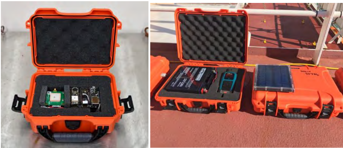
Figure 2-2 (a) Cryologger iceberg tracking beacon; (b) Cryospheric iceberg tracking beacon (Rockstar Iridium)
