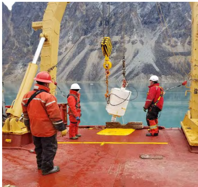
Figure 26-2 Piston coring in Coronation Fjord, Baffin Island.
