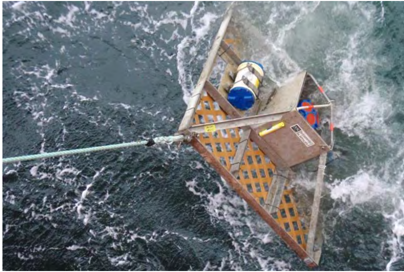
Figure 7.10. Recovery of ASL/IOL-BP bottom frame mooring at site C (Photo: ASL Cruise Report 2009).
