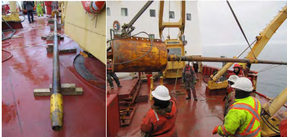
Figure 36.4. Preparation and deployment of the piston core used for geotechnical sampling during Leg 3b.
