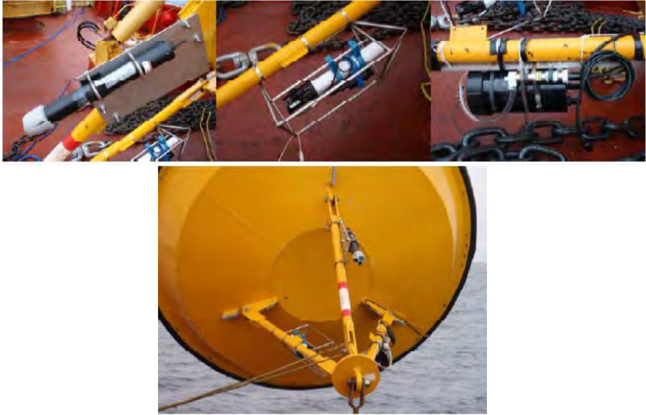
Figure 3.4. Underwater instrumentation associated with the Met/Ocean buoy. Nortek® Aquadopp surface current meter (left), RBR® multi-probe (middle) and Pro-Oceanus® pCO 2 -pro (right) installed on the anchor yoke (lower panel). Sensor specifics appear in Table 3.4 and 2.5. Photos: E. Stainton and IOL.
