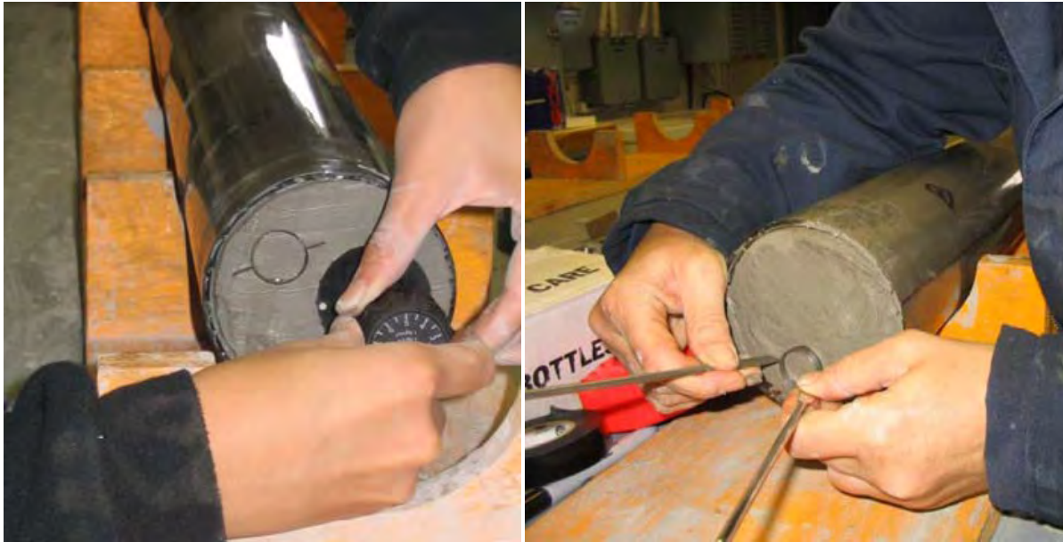
Figure 36.7. Left: Shear strength measurements performed on the sediment cores collected during Leg 3b. Right: Bulk density and water content determinations conducted on cores collected during Leg 3b.
