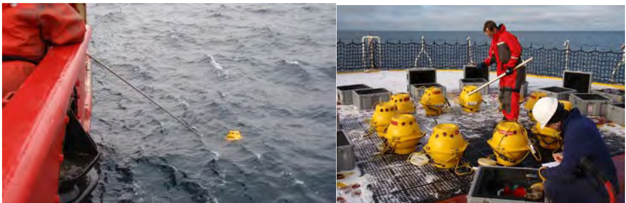
Figure 32.4. Left: Retrieving the MARU from the foredeck during Leg 3b, and right: time synchronization of MARU buoys on the flight deck of the Amundsen .
