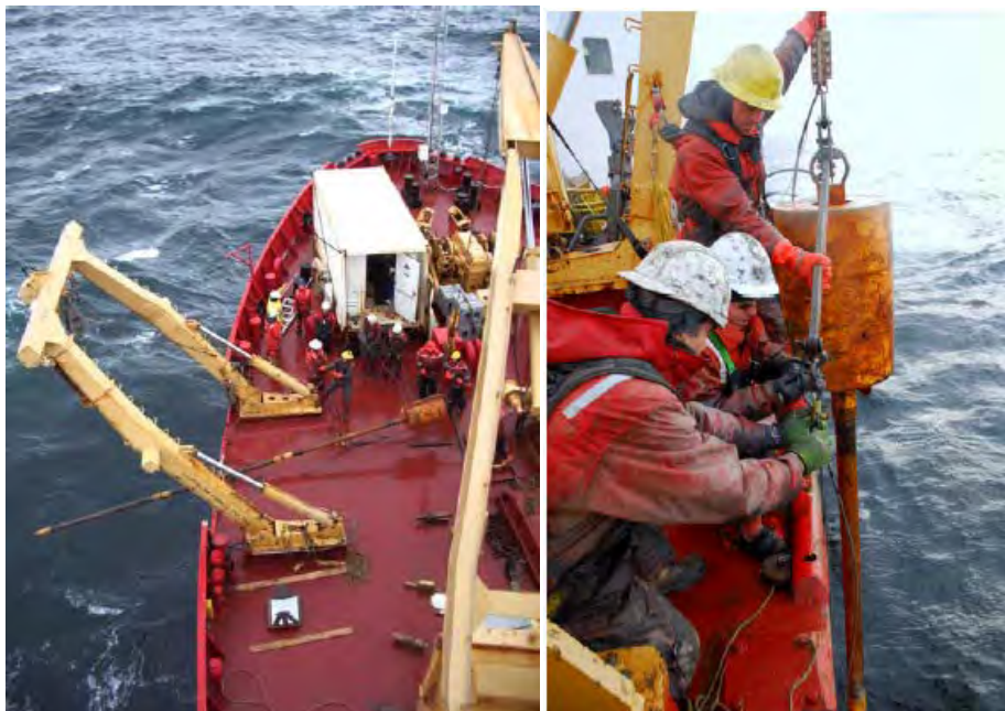
Figure 36.6. Deployment of the piston core or Trigger Weight Core (TWC) from the foredeck during Leg 3b.
