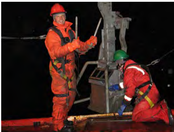
Figure 37.1. Recovery of the box corer used to sampled endofauna and sediments.
