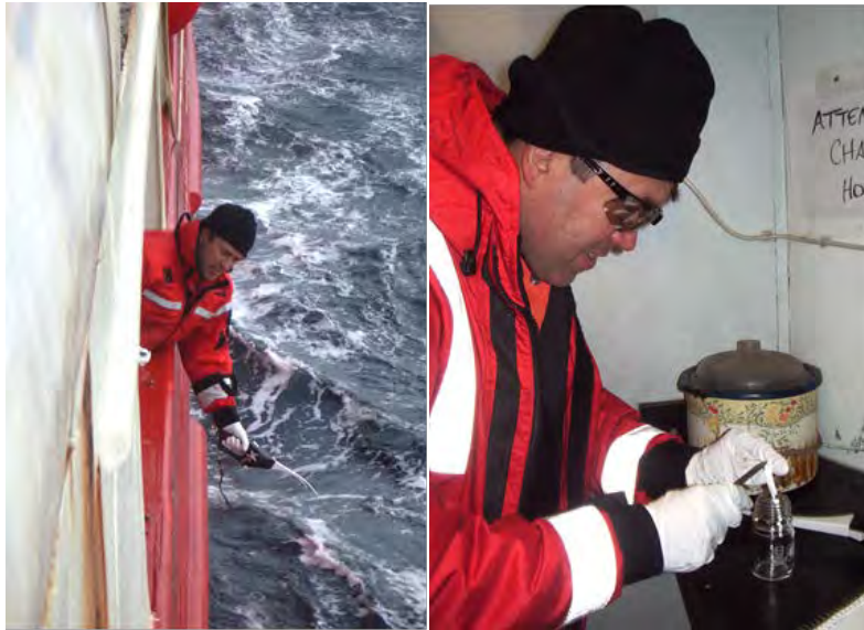
Figure 36.9. Deployment and processing of the GORE surface oil slick samplers used during Leg 4a.
