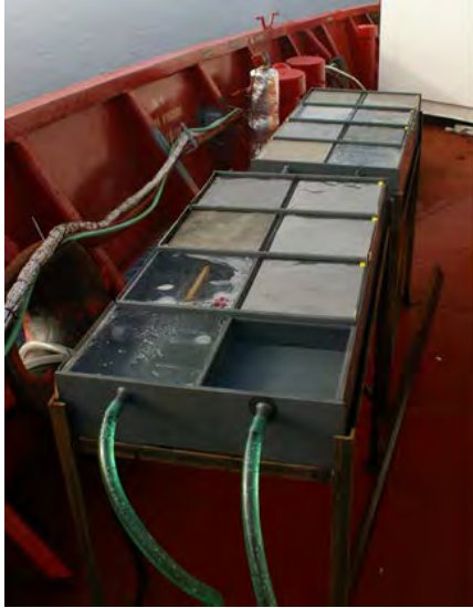
Figure 27.1. Incubation basins flowing with seawater and simulating different light levels (100%, 50%, 25%, 15%, 8%, 3%, 1%) were used for production rate experiments during Leg 2a.
