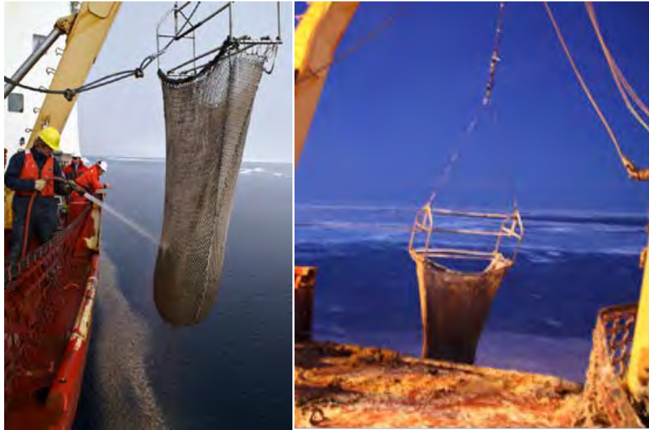
Figure 37.3. Agassiz trawl used to collect benthic epifauna.
