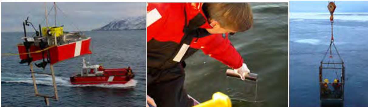
Figure 4.1. Microlayer sampling techniques used during Legs 4a and 4b: Left: Little Kilo Moana during deployment from the CCGS Amundsen , Middle: glass plate sampling (at Saanich Inlet, BC) and Right: sampling from the ice cage deployed from the Amundsen .
