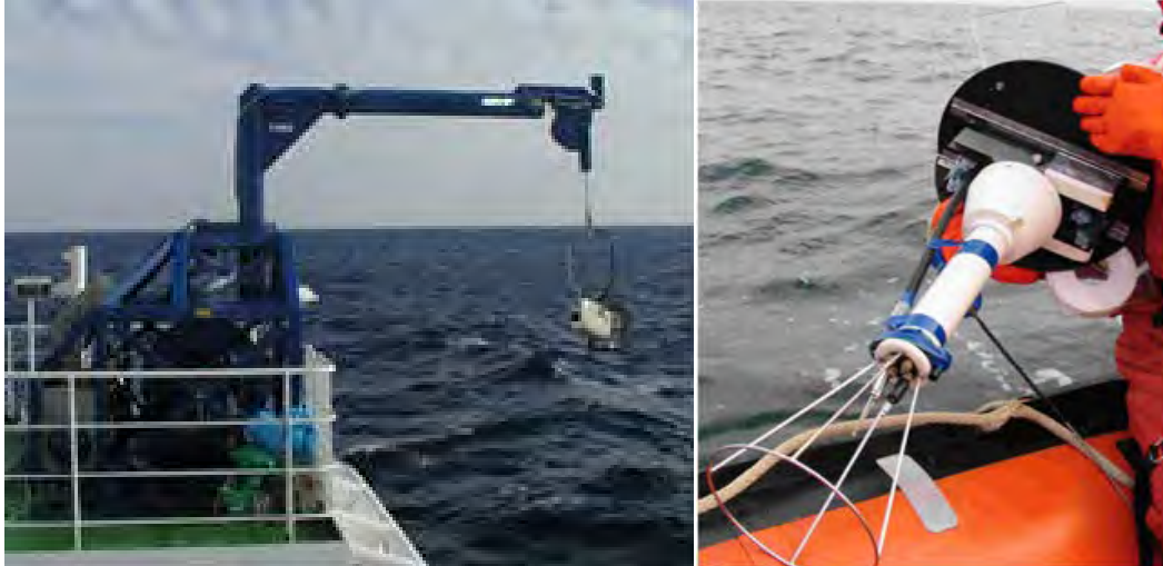
Figure 10.1. Left: The Moving Vessel Profiler (MVP) being deployed. Right: The SCAMP profiler used during Leg 2b.
