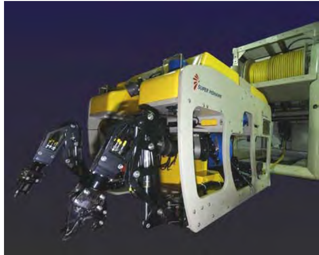
Figure 35.2. The CCGS Amundsen 's Sub-Atlantic Super Mohawk Remotely Operated Vehicle (ROV).
