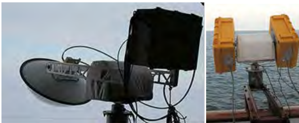
Figure 5.4. Left: Scatterometer, Right: Passive microwave radiometers (SBR) (37 and 89 GHz) installed on port side of the Amundsen ~10 m above sea level.
