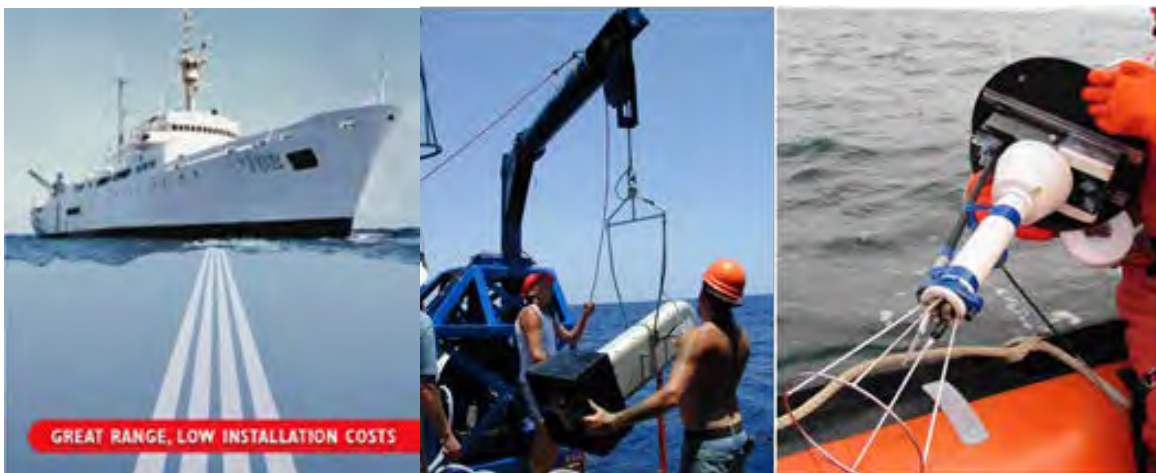
Figure 9.2. The SM-ADCP (Ship-Mounted Acoustic Current Profiler; left), the MVP (Moving Vehicle Profiler; center) and the SCAMP (Self-Contained Autonomous Micro-Profiler; right) used on the Amundsen .
