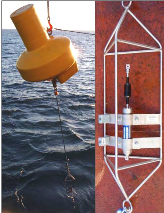
Figure 7.13. Uppermost Alec EM current meter in-line beneath one of the secondary surface buoys accompanying the MetOcean AXYS® buoys (ASL Cruise Report Leg 3b, 2009).
