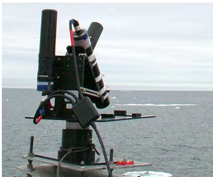
Figure 5.11. The HyperSAS instrument mounted on the bow of the CCGS Pierre Radisson during the BaySys cruise in Hudson Bay in July and August 2009.
