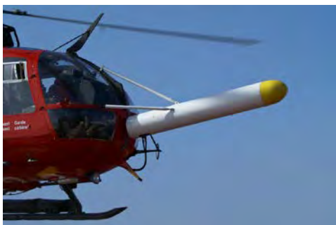
Figure 5.3. EM induction system mounted on the front of the helicopter.
