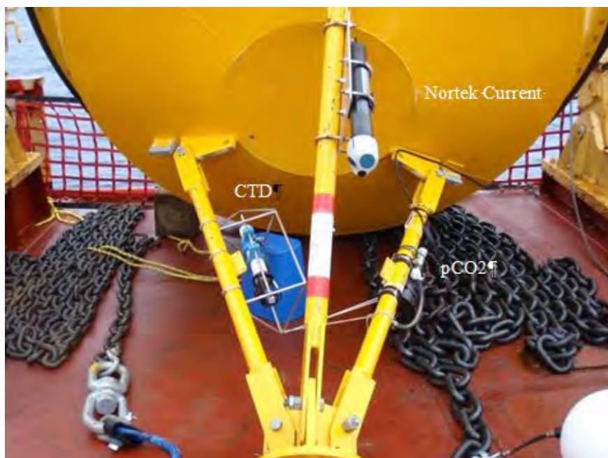
Figure 7.12. The three instruments mounted beneath the 3 m MetOcean AXYS® buoy deployed at Site A1: RBR CTD, Nortek Current Profiler & the Pro-Oceanus pCO 2 .
