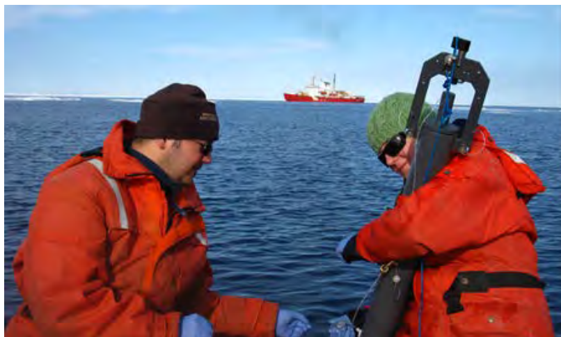
Figure 33.2. Surface sample collection using the Zodiac and a Niskin bottle.
