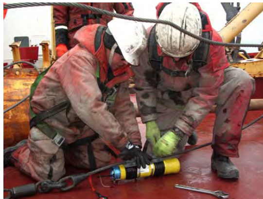
Figure 36.5. USBL beacon attached above the piston core head prior to deployment.
