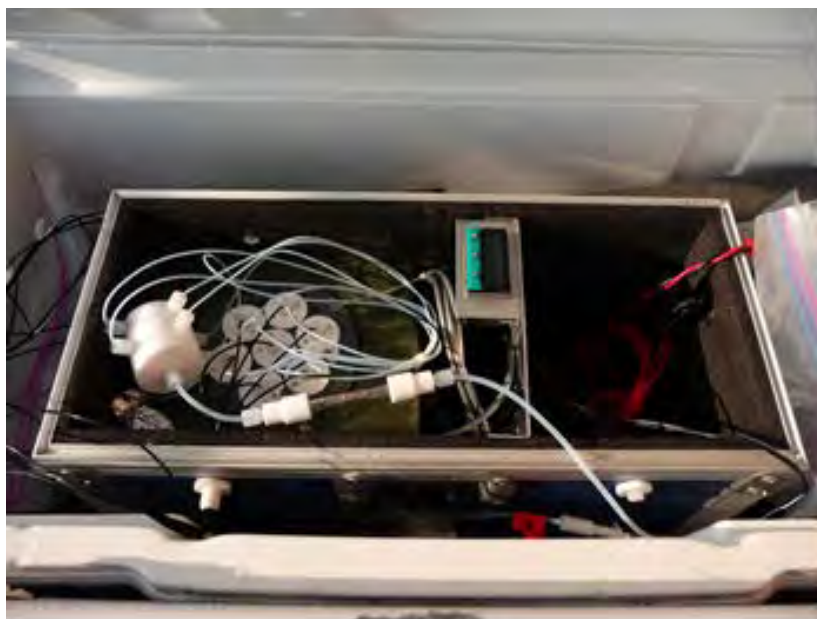
Figure 2.3. Mercury permeation system used for atmospheric measurements in Legs 1b and 4a.
