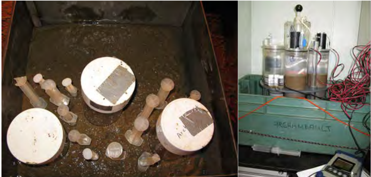
Figure 37.2. Left : Box core with upper half for diversity/abundance sieving and lower half for SOD/Nutrient cores (white caps), pigment concentration cores and Meiofauna samples (big syringes), CN cores and bacteria samples (medium syringes) and Meiofauna/Microfauna incubation samples (small syringes). Right : Incubation setup in the temperature controlled room with SOD cores, mini-incubations and the Fibox optical oxygen probe.
