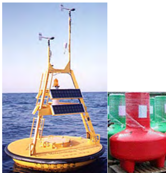
Figure 7.11. ArcticNet MetOcean-AXYS® oceanographic buoy (3m diameter) and surface buoy (red – right) deployed at mooring site A1-09 (size relative to each other).
