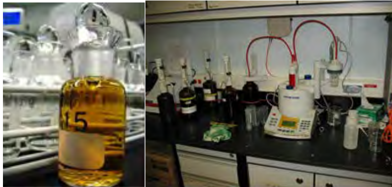
Figure 9.5. Bottles used to collect samples (left) for oxygen calibration and the Mettler Toledo titrator (right) used to analyze the samples onboard the Amundsen .
