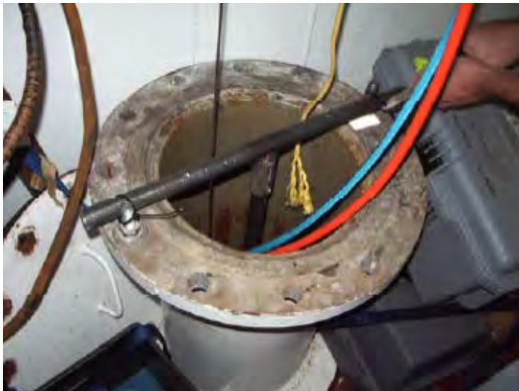
Figure 36.3. USBL calibration beacon deployed through the ship's acoustic well before the start of coring and ROV operations.
