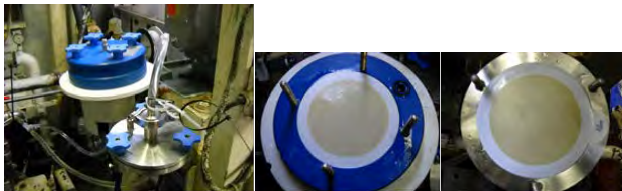
Figure 25.1. Left: Underway filtration unit in the engine room. Middle: Underway filtration setup for biomarker analyses (GF/F filters). Right: Underway filtration setup for Si isotopes (Supor filters).
